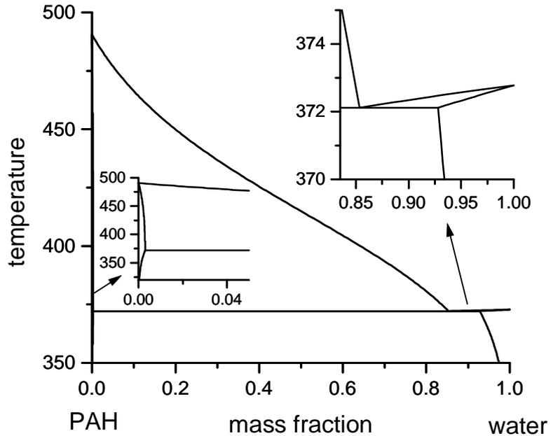
Fig. 3. Constructed phase diagram of naphthalene-water
