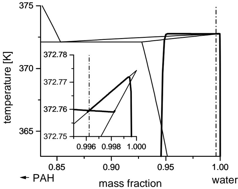
Fig. 4. Dynamics of the stripping in phase diagram, Fig. 3. Thick curves correspond to droplet and vapour at surface temperature. Dot-dashed line – total mass fraction  $x_t$  in cell
