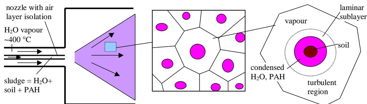
Fig. 1. Spraying of the sludge added by superheated steam and steam stripping of PAH contaminated droplets
