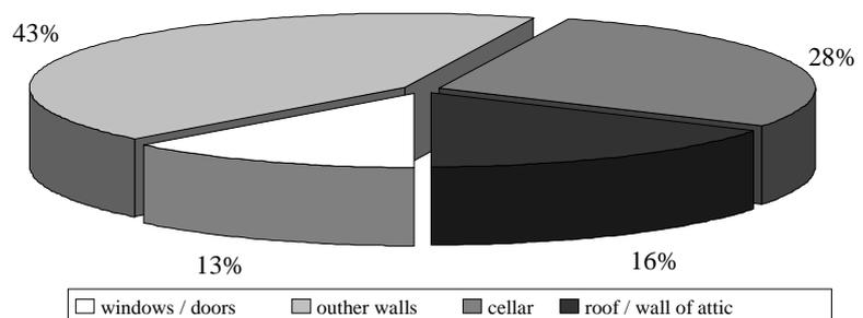
Fig. 2. Constitution of areas of elements in heated part of the outer shell of building
