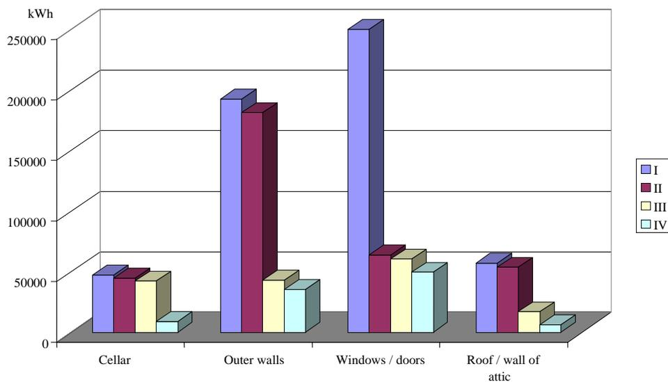
Fig. 7. Annual constitution of heat losses through the elements of the outer shell of building
