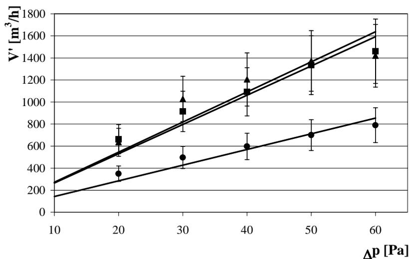
Fig. 1. Air flux vs. pressure difference for buildings with various degrees of packing.
