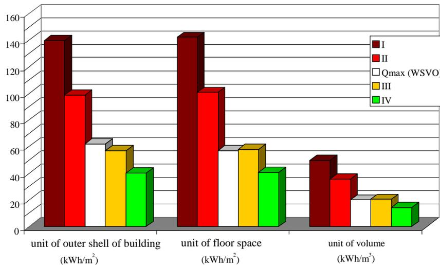
Fig. 3. Comparison of normalised heat consumption with respective marginal values of building normatives in Germany.
