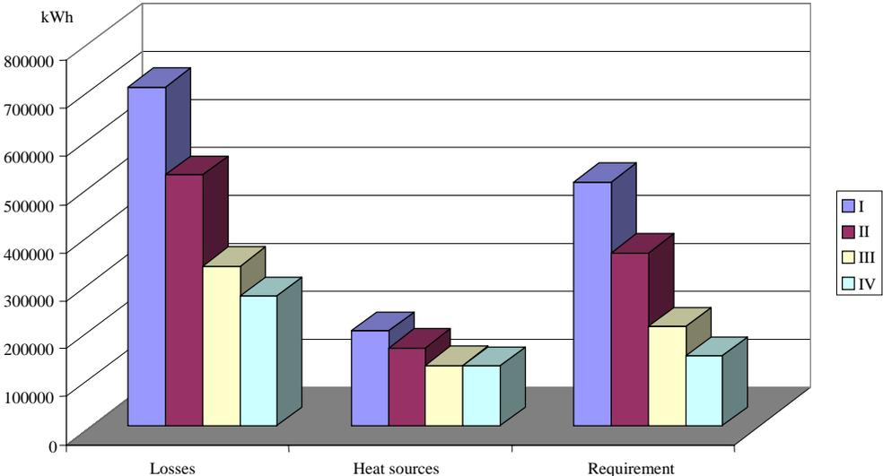
Fig. 4. Normalised annual heat consumption of building in initial state (I) and various variants of renovation (II, III, IV)
