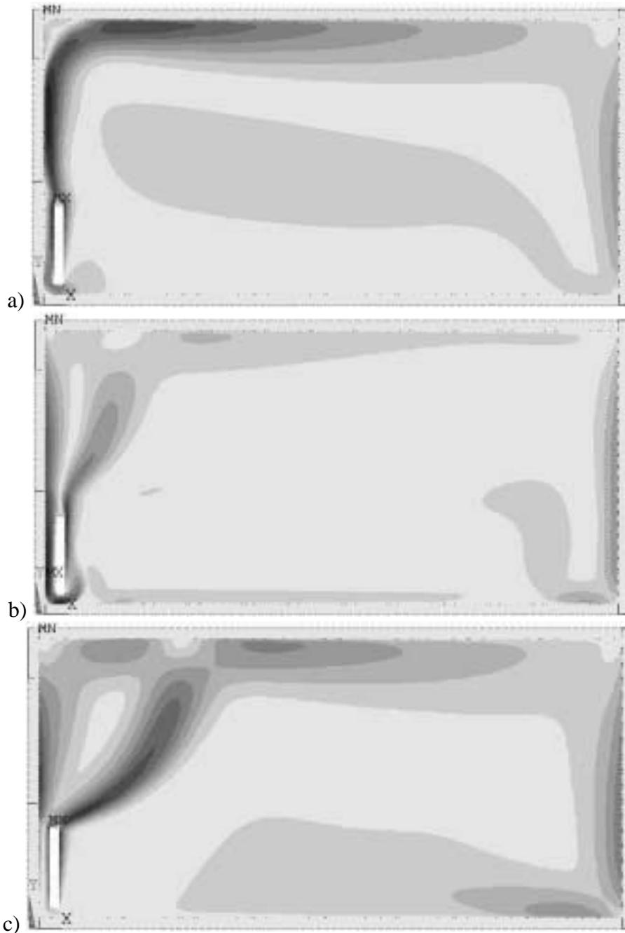
Fig. 2. Stationary distribution of the module of velocity in the room. a, b, c correspond to variants 1, 3, 4, respectively.
