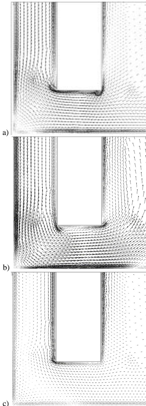
Fig. 5. Air flux pattern below the heater. a, b, c correspond to variants 1, 3, 4, respectively.
