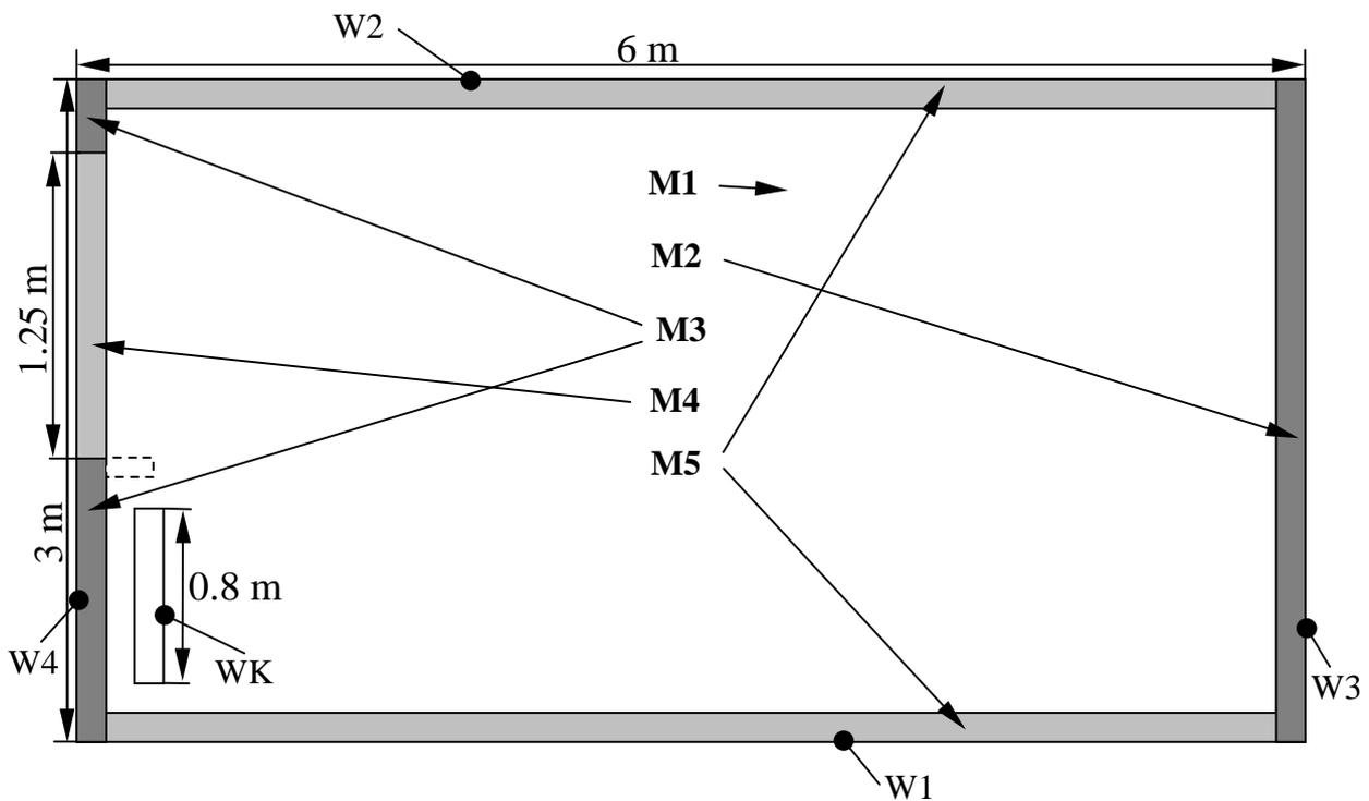
Fig. 1. Layout of building elements in modelled room
