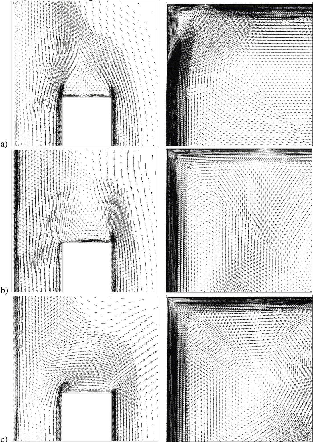
Fig. 3. (left) Air flux pattern above the heater. a, b, c correspond to variants 1, 3, 4, respectively.
