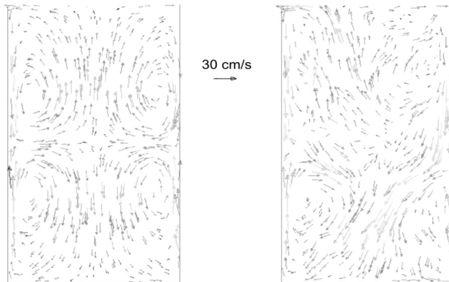
Fig. 7 and 8. Calculated with LES turbulence model flow pattern with symmetric dominating flow eddies and after 30 seconds of transient simulation with the time-step 10ms
