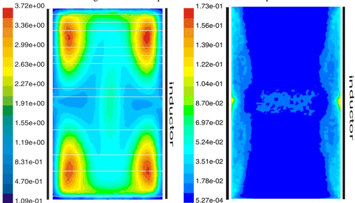
Fig. 2 and 3. Characteristic turbulent viscosity distribution in [kg/m·s] calculated with 3D k-ε and LES turbulence models
