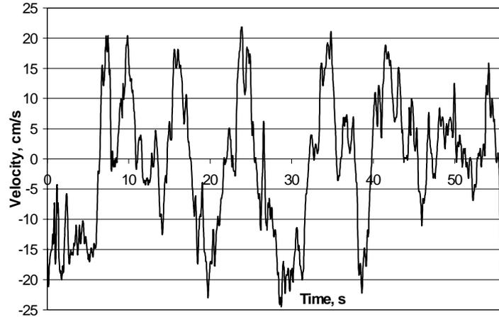
Fig. 1. Axial velocity oscillations measured in experimental ICF in the region between the dominating flow eddies near the crucible wall
