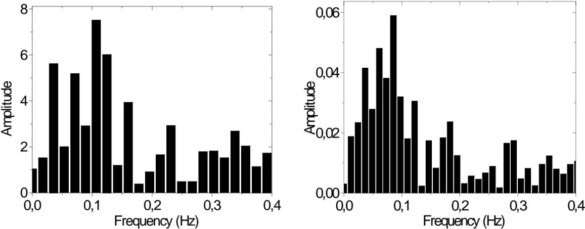
Fig. 5 and 6. Fourier analysis of the measured (left) and calculated with 3.5 mil. elem., time-step 10 ms (right) oscillation of the axial velocity components near the crucible wall at half-height of the inductor. Amplitudes are in [cm/s] on the left and in [m/s] on the right graph.
