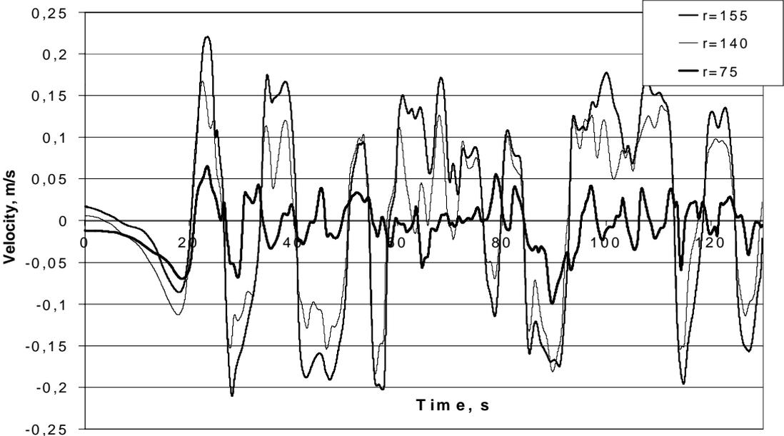
Fig. 4. Axial velocity oscillations at the middle-height of the inductor calculated with 3D LES turbulence model (mesh contains 400 thousands elements)
