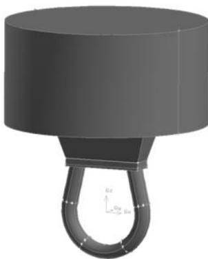
Fig. 1. Original design of ICF with symmetrical channel
