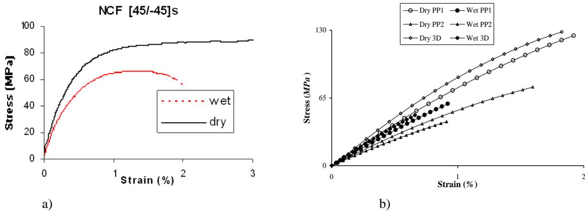
Fig. 2. Moisture effect on stress-strain curves of a) NCF; b) PP1, PP2 and 3D composites
