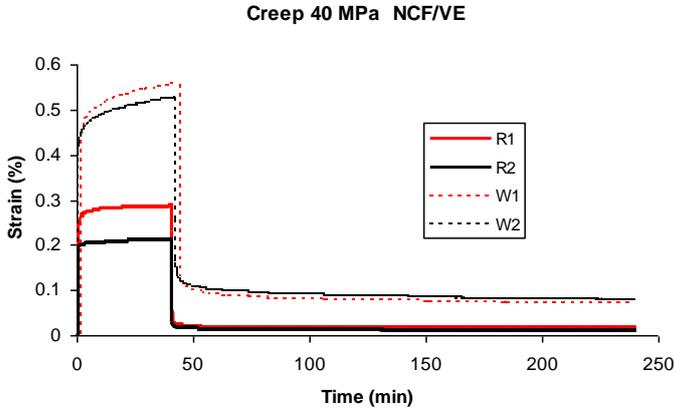
Fig. 3. Creep curves at 40 MPa applied stress for reference(dry) and wet NCF composite. W is notation for wet specimen, R –for dry reference specimen
