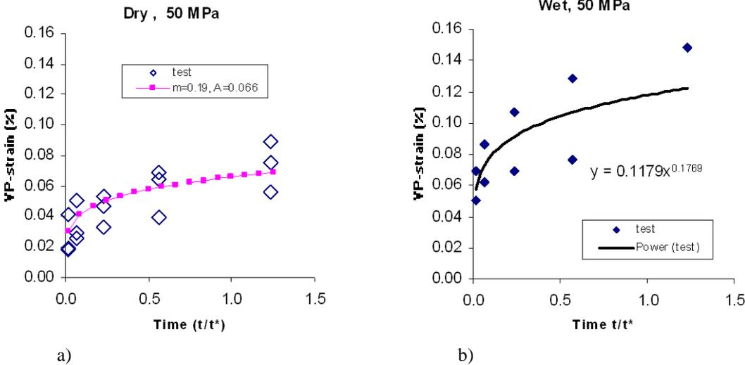
Fig. 4. Viscoplastic strain accumulation in NCF composite during creep test at 50 Mpa: a) dry specimens; b) wet specimens. Fit to data is shown as solid line. Characteristic time  $t^*=3600$  sec
