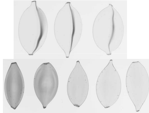
Fig. 2. Glass flakes obtained in experiment. Above – no EM mixing, flakes obtained with 10 min difference, below – with EM mixing
