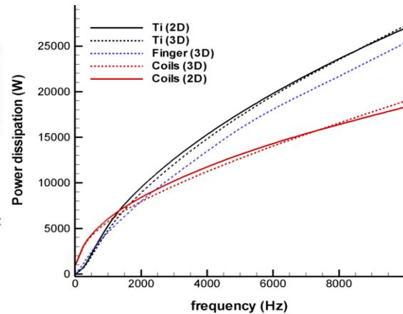
Fig. 4. Power dissipation in conducting regions as a function of frequency when  $I_{eff}=5 kA$
