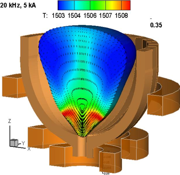
Fig. 7. The velocity field and temperature distribution in the magnetically levitated liquid titanium after several seconds of the flow and shape adjustment to a quasi-stationary shape computed by the SPHINX model
