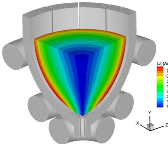
Fig. 1. One quarter of the crucible showing  $|\mathbf{J}|$  in the titanium computed with COMSOL; coil current  $I_{\text{eff}}=5$  kA,  $f=2$  kHz
