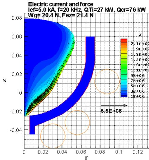
Fig. 5. Axisymmetric solution showing  $|\mathbf{J}|$  and the force distribution in the hemi-spherical titanium at initial time moment; coil current  $I_{\text{eff}}=5 \text{ kA}$ ,  $f=20 \text{ kHz}$
