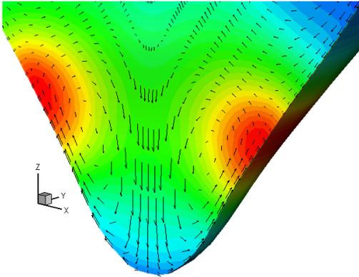
Fig. 8. The zoom-in to the velocity field at the bottom part of the magnetically levitated liquid titanium in a quasi-stationary shape
