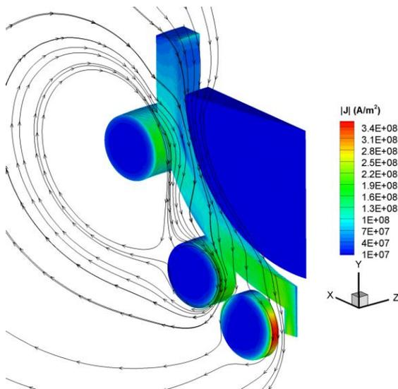
Fig. 3. Model showing (i) 3D streamlines of magnetic flux squeezing through the space between the fingers and (ii) scalar plot of  $|\mathbf{J}|$  with  $I_{eff}=5kA$  and  $f=2kA$  (due to symmetry only half a finger/air gap is considered)
