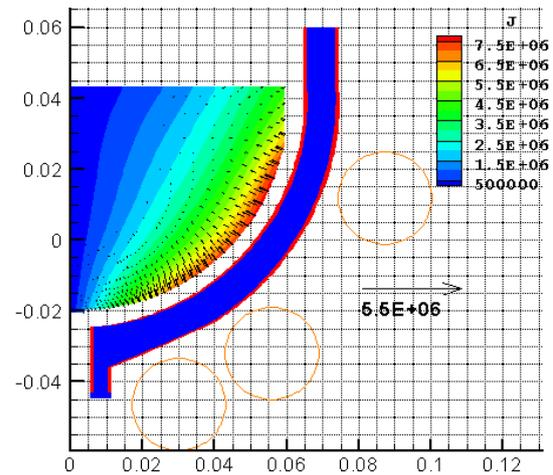
Fig. 2. Axisymmetric solution showing  $|\mathbf{J}|$  and the force distribution in the titanium computed by the SPHINX model; coil current  $I_{\text{eff}}=5$  kA,  $f=2$  kHz
