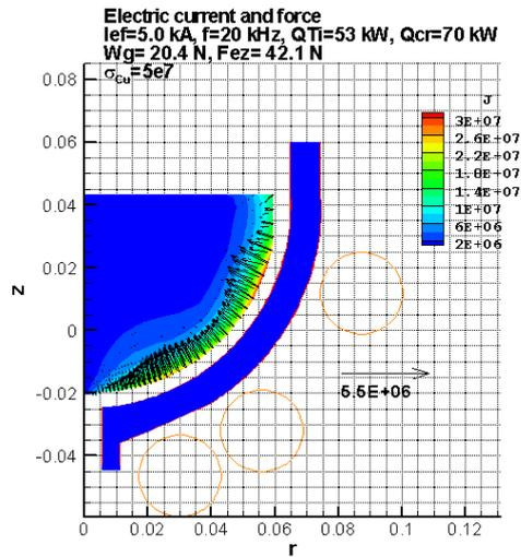
Fig. 6. Axisymmetric solution showing  $|\mathbf{J}|$  and the force distribution in the magnetically levitated liquid titanium after several seconds of the flow and shape adjustment to a quasi-stationary shape computed by the SPHINX model; coil current  $I_{\text{eff}}=5 \text{ kA}$ ,  $f=20 \text{ kHz}$
