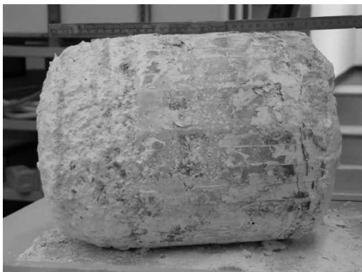
Fig. 2. Ingot in the “big” cold crucible was produced which is partly composed of single crystals of 50 mm length. The huge ingot taken out of the cold crucible is shown in Fig. 2.
