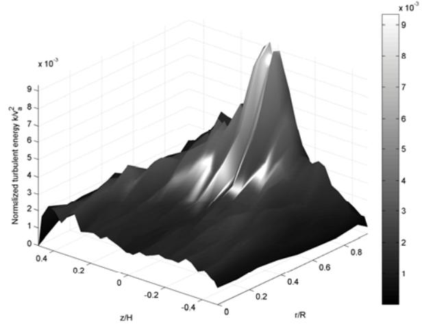
Figure 2. Experimental distribution of the normalized averaged axial pulsation kinetic energy  $k/v_A^2$  ( $I = 2000$  A,  $f = 395$  Hz,  $B_0 = 0.098$  T,  $v_A = v_{Alfven} = 0.9$  m/s).
