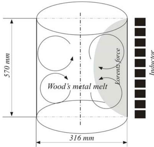
Figure 1. Design of laboratory CIF with sketch of typical vortices of the mean flow.
