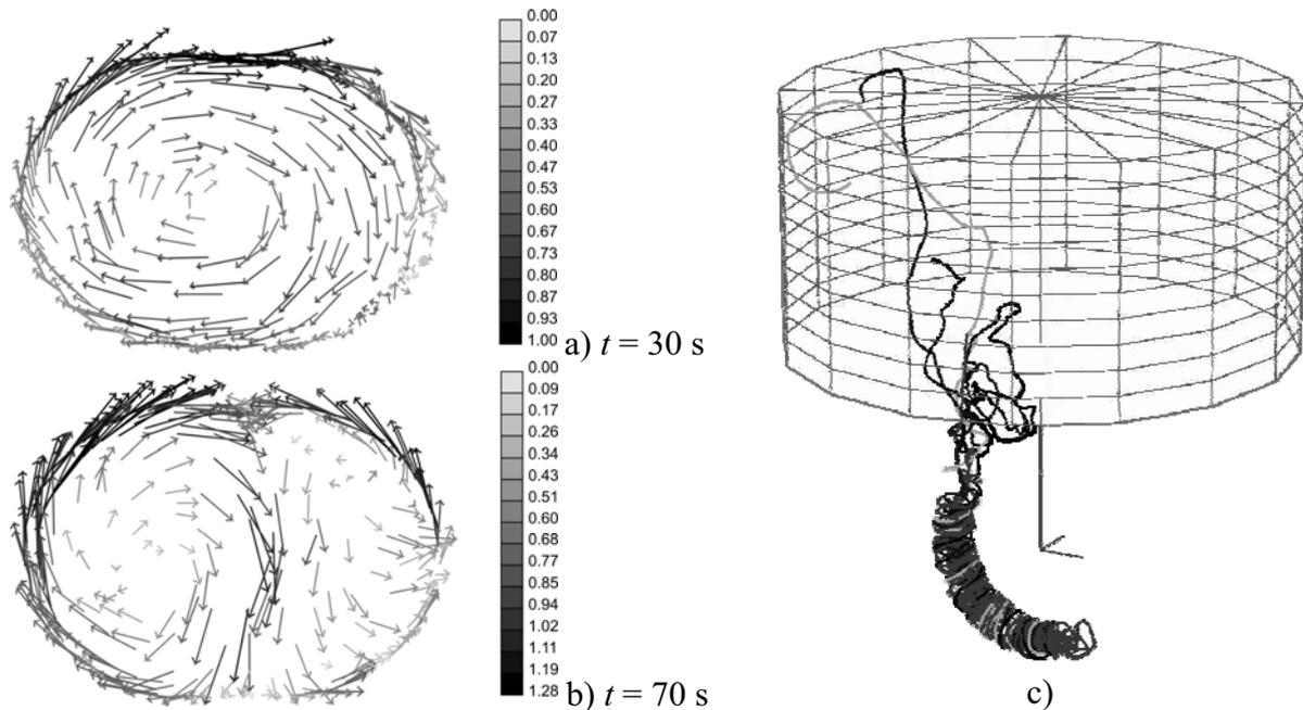
Figure 5. LES calculated instantaneous velocities in the channel cross-section of 300 kW ICF and 50 s tracks of 0.2 mm particles ( $\sigma_p = 0$ ,  $\rho_p \approx 0.75\rho = 5250 \text{ kg/m}^3$ ).
