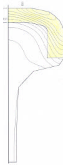
Fig. 4: Partial heater for railway tracks and temperature distribution in the head
