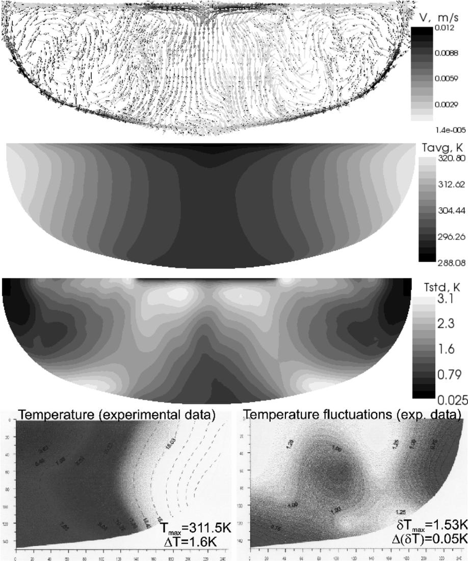
Fig. 1. 3D LES calculations with Smagorinsky model and van Driest damping for crucible rotation -5 rpm and crystal rotation 15 rpm. From top to bottom: averaged velocity, temperature, and root mean square temperature fluctuation distributions, experimental averaged temperature and its fluctuations distributions.
