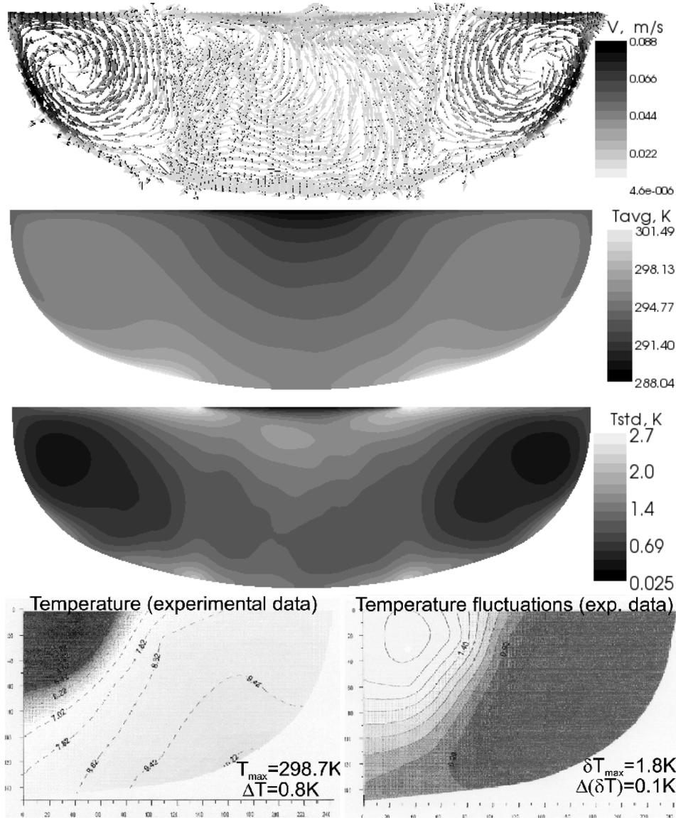
Fig. 2. 3D LES calculations with Smagorinsky model and van Driest damping for crucible rotation -5 rpm and crystal rotation 15 rpm and TMF „down”. From top to bottom: averaged velocity, temperature, and root mean square temperature fluctuation distributions, experimental averaged temperature and its fluctuations distributions.
