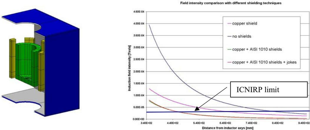
Figure 5: Schematic of different shielding solutions and values of magnetic flux density along a radial line from the center of the inductor
