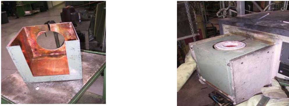
Figure 6: The real shield and the implementation on the induction furnace
