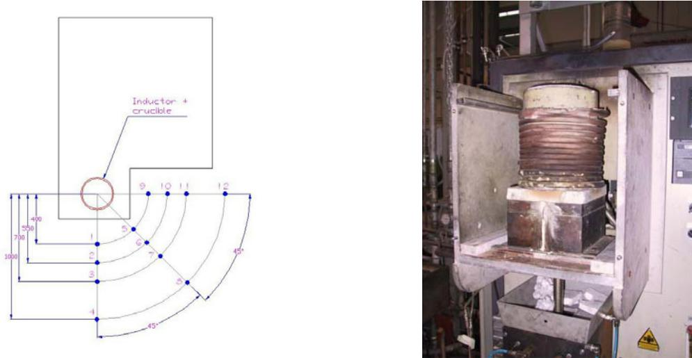
Fig 1: on the left the schematic of the furnace and points where the measurements have been done; on the right a picture of the furnace inductor
