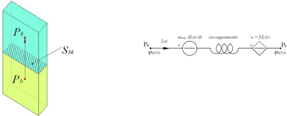
Figure 4: a particular of the mesh and the circuit model associated to it
