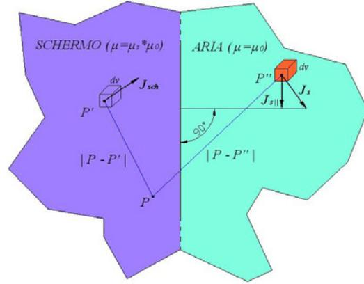
Figure 3: Evaluation of the magnetic vector potential A at the point P as contribution of primary and secondary sources
