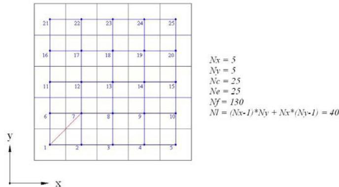
Figure 2: Example of discretization of shielding sheet used for the integral method
