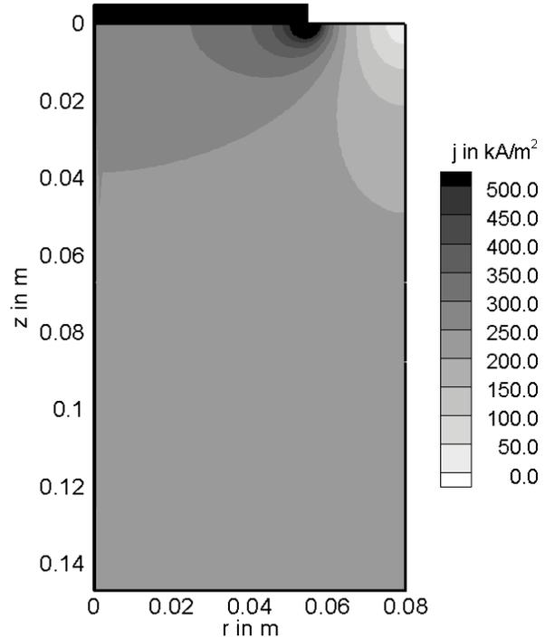
Fig. 3: Current density distribution without motion of the steel-slag interface
