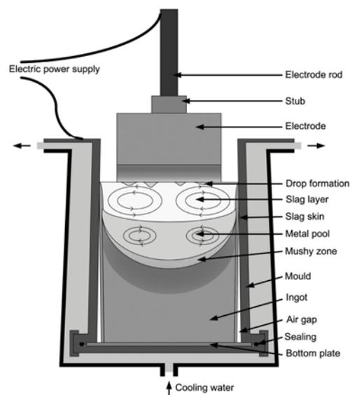
Fig. 1: Design of an ESR plant
