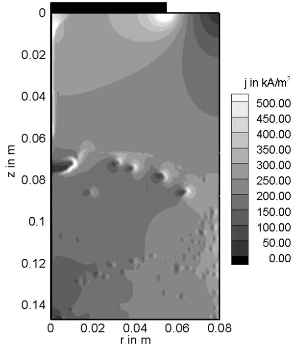
Fig. 5: Current density distribution with droplet movement
