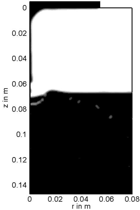
Fig. 4: Slag and steel fraction with droplet movement
