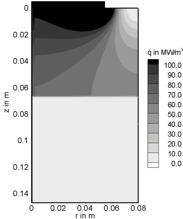
Fig. 2: Heat input due to Joule heating without motion of the steel-slag interface
