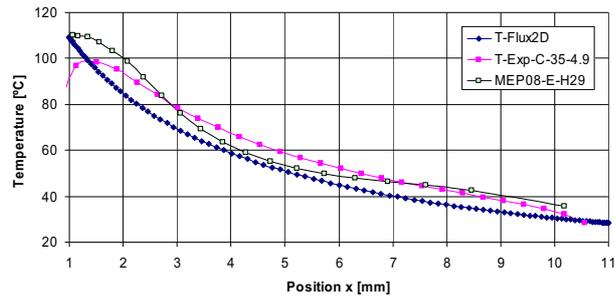
Fig. 5. The left part of the figure shows the isotherm on the cross section of the tube (30 to 100 °C in steps of 10 °C from right to left). The graph shows the temperature on the upper surface of the tube as a function of position x; Numerical and experimental with camera straight above coil and with camera at an angle sideways.
