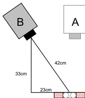
Fig. 3. Thermographic camera positions. A-Old B-New
