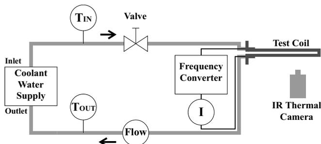
Fig. 2. Experimental setup. Gray lines are coolant and black lines electricity.
