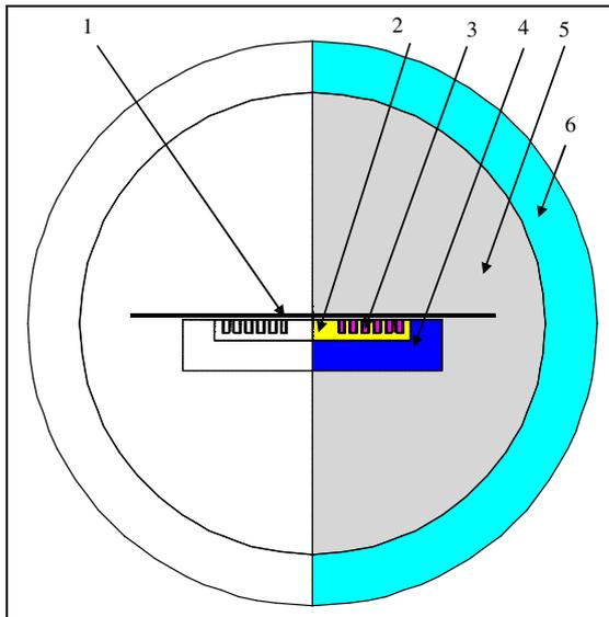
Fig. 2. Magnetoforming of flat sheets – 2D computation domain: 1-metallic sheet; 2-electric insulation; 3-forming coil; 4-magnetic shield; 5-air; 6-“infinite” region
