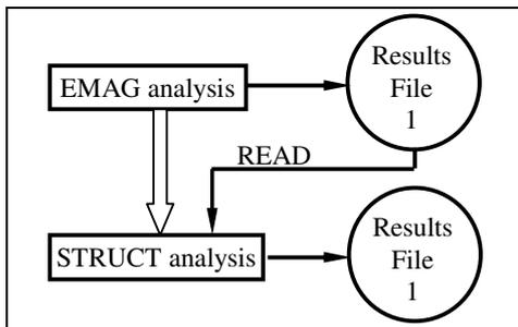
Fig. 3. One step in sequential coupling in an electromagnetic – structural coupled problem solving.
