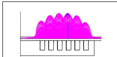
At each time step, electromagnetic simulation gives at each finite element the volume density of electromagnetic force. These force vectors in the sheet region are depicted in Fig. 5. The model is built in ANSYS Multiphysics 10. The computation domain for electromagnetic problem and the corresponding mesh is shown in Fig. 7, in which the 2D 8 nodes quadrilateral
