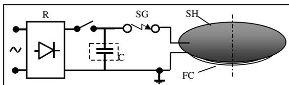
Fig. 1. EMF facility for forming metal sheets:
