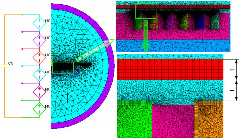
Fig.7. The computation domain and mesh in ANSYS model.
