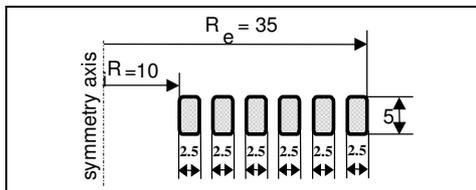
Fig.4 The geometry of the forming coil
