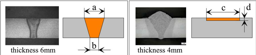
Fig. 1. Principles of laser and GMA welding energy implementation
