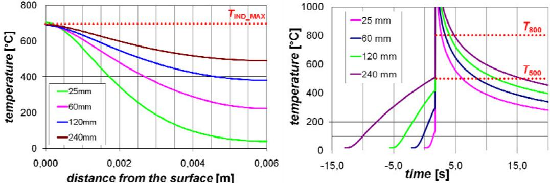
Fig. 4. Laser welding process with induction preheating: influence of the length of coil (left: temperature profile over the sheet thickness; right: time-temperature distribution on the root side of the weld)
