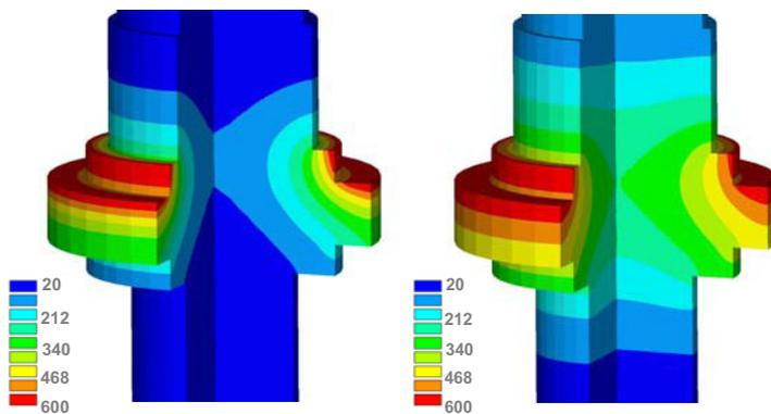
Fig. 7. Temperature distribution after 50 s (left) and after 100 s (right) of preheating
