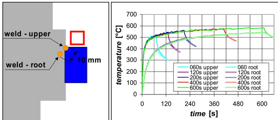
Fig. 8. Sketch of the arrangement with observed points in the welding zone (left); time-temperature distribution on the root and upper side of the weld for different pre-heating times (right)
