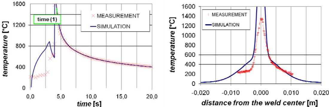
Fig. 3. Time-temperature distribution on the upper side of the weld and temperature profile on the upper side after the laser process for time (1)
