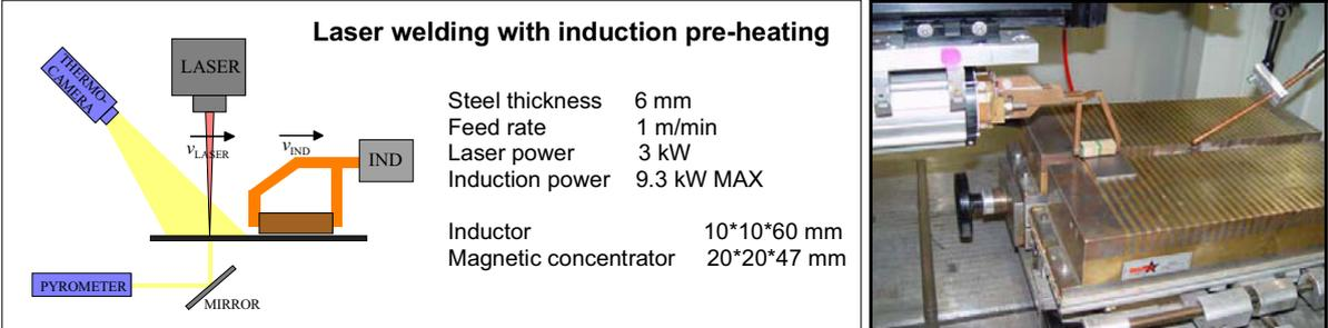
Fig. 2. Parameters of the investigated process and overview of the experimental installation (IWS Dresden)
