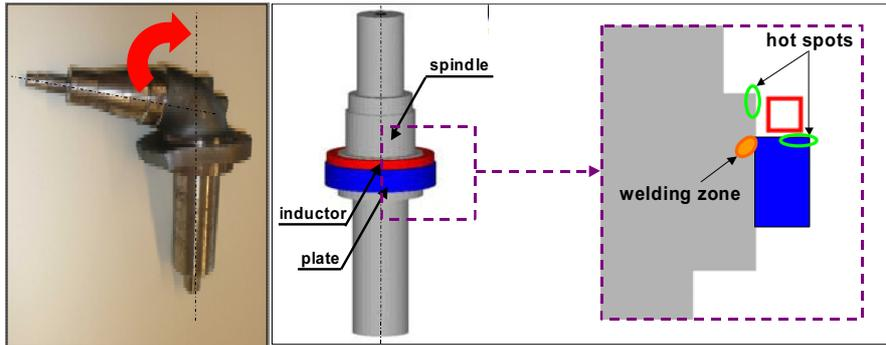
Fig. 6. Welded parts (produced by CNH Belgium N.V.) and schematic sketch of investigated welding arrangement
