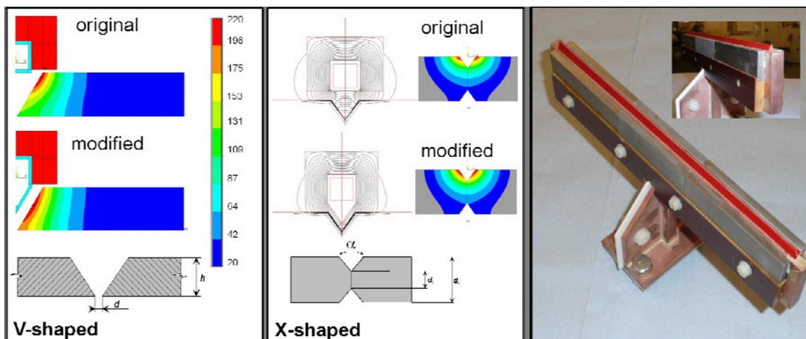
Fig. 5. Induction pre-heating: Influence of inductor geometry on temperature profile and photograph of the experimental inductor
