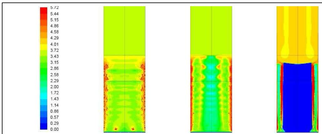
Fig. 1. Averaged concentration at  $t=2500s$ . Left  $B=5mT$ , middle  $B=10mT$ , right  $B=30mT$ . The flow is upward to the sides. The horizontal lines corresponds to the coordinates  $z=1cm$  and  $z=1.5cm$
