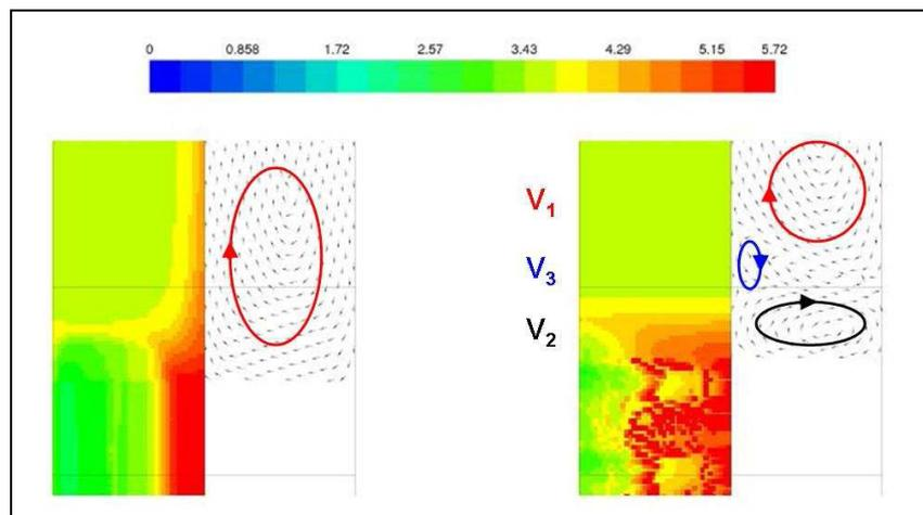
Fig. 3. Averaged concentration and flow pattern for  $B=5mT$  at  $t=2500s$ . Left: without buoyancy effect. Right: with buoyancy effect. The horizontal lines correspond to the coordinates  $z=1cm$  and  $z=1.5cm$ .
