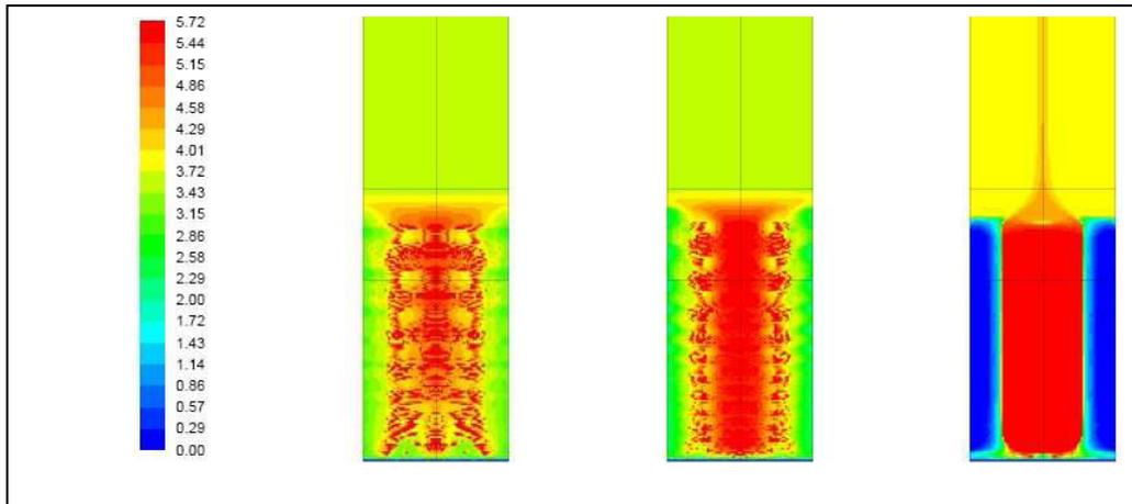
Fig. 2. Averaged concentration at  $t=2500s$ . Left  $B=5mT$ , middle  $B=10mT$ , right  $B=30mT$ . The flow is upward to the middle. The horizontal lines corresponds to the coordinates  $z=1cm$  and  $z=1.5cm$
