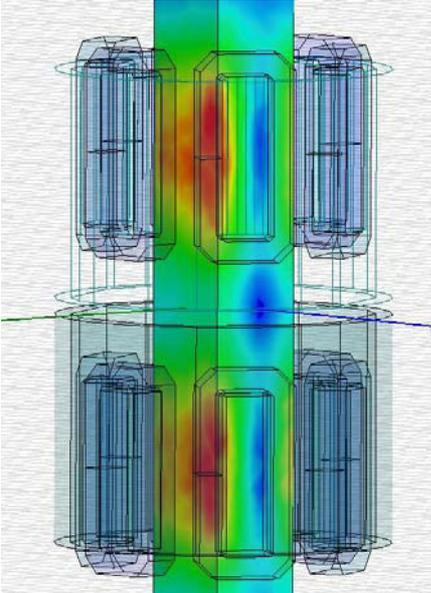
Fig. 5. Typical current distribution on strand surface.
