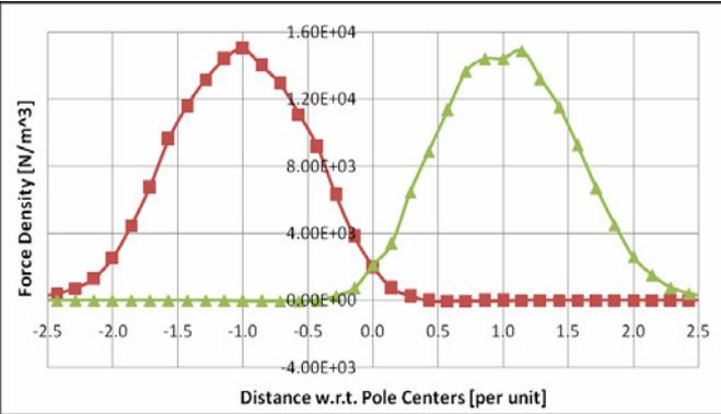
Fig. 2. Typical force distributions due to two axially displaced stirrers acting separately.
