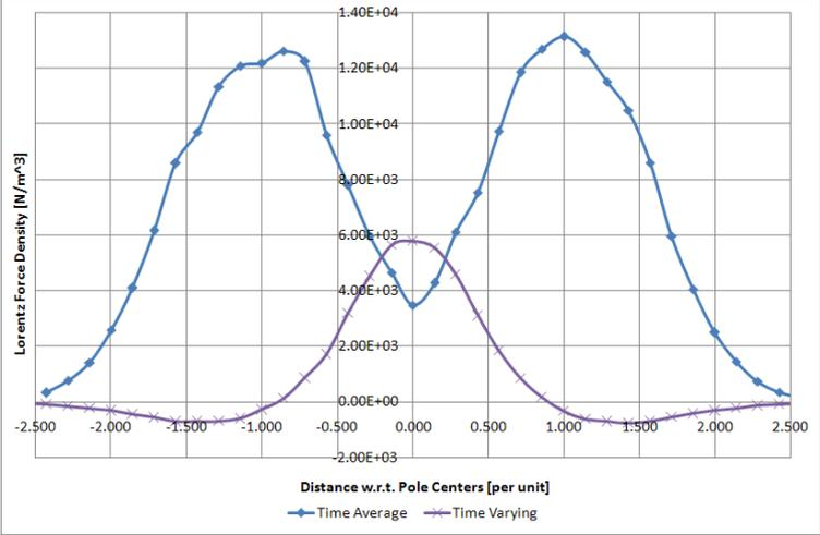
Fig. 6. Representative Lorentz force distributions within molten core - time average plus low frequency time varying.
