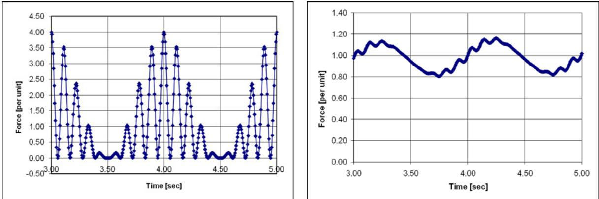
Fig. 4a (left). Actual modulated force due to the interaction of two adjacent stirrers, including DC, low frequency and high frequency terms.
