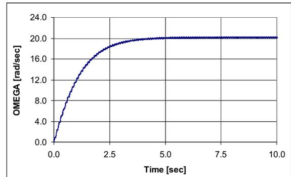
Fig. 3. Transient response of a cylindrical strand to a 1000 Gauss magnetic field rotating at 5 Hz.
