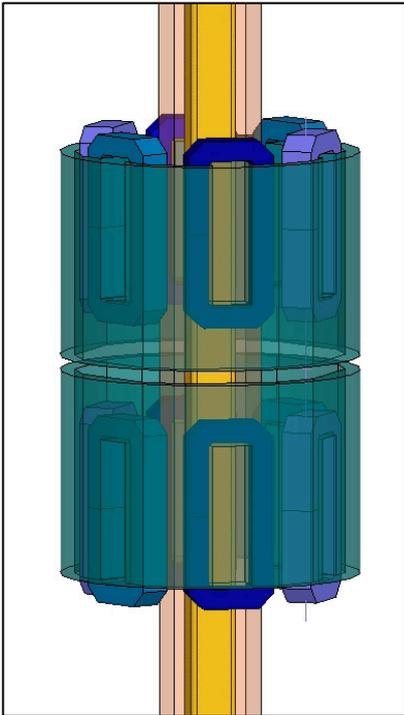
Fig. 1. Dual EMS system for advanced solidification zone stirring.
