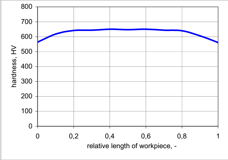
Fig.5 Hardness distribution along working plane of the tool
