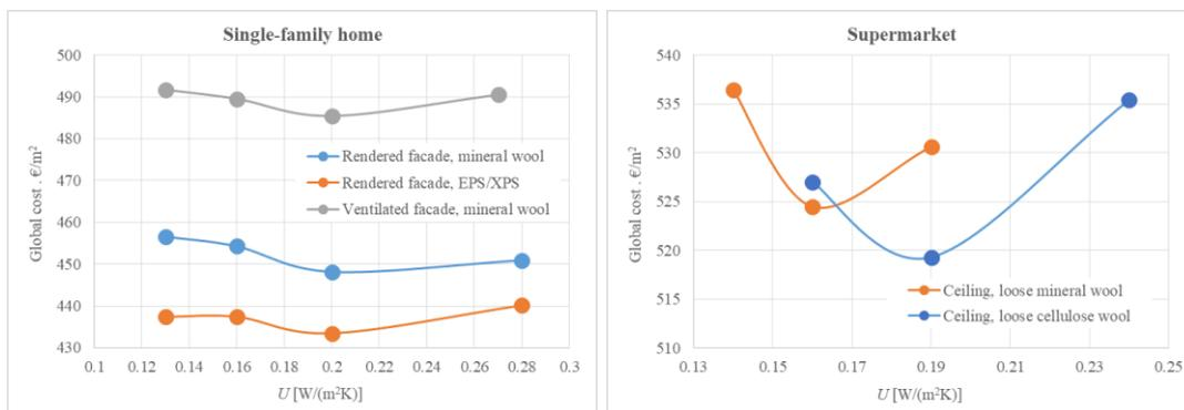
Fig. 4. Cost-optimal  $U$ -value for facade and ceiling insulation with different materials.
