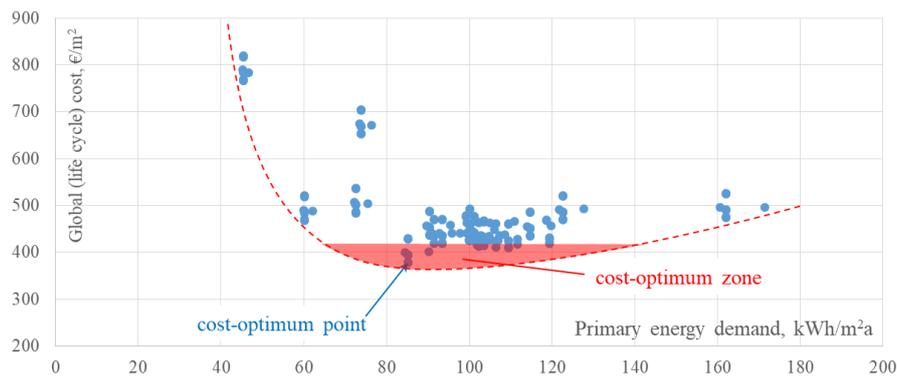
Fig. 1. Example of graphical representation of cost-optimum measures.
