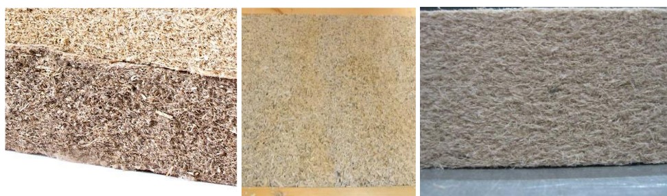
Fig. 4. Hemp batts (left), hemp-lime concrete (centre), and wood fibre (right).
