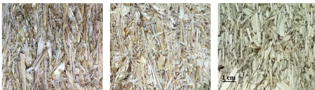
Fig. 3. Fibres of pressed rye (left), reed straw (centre), and hemp shives (right).
