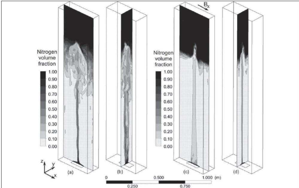
Fig. 2.  $N_2$ -Wood-metal RBR – cross-sections: (a, c)  $y=0$  and (b, d)  $x=0$ . Instantaneous (flow time  $t = 5$  s) contours of nitrogen volume fraction: (a, b) without magnetic field  $B = 0$ ; (c, d) with transversal external magnetic field  $B_x = 0.1$  T
