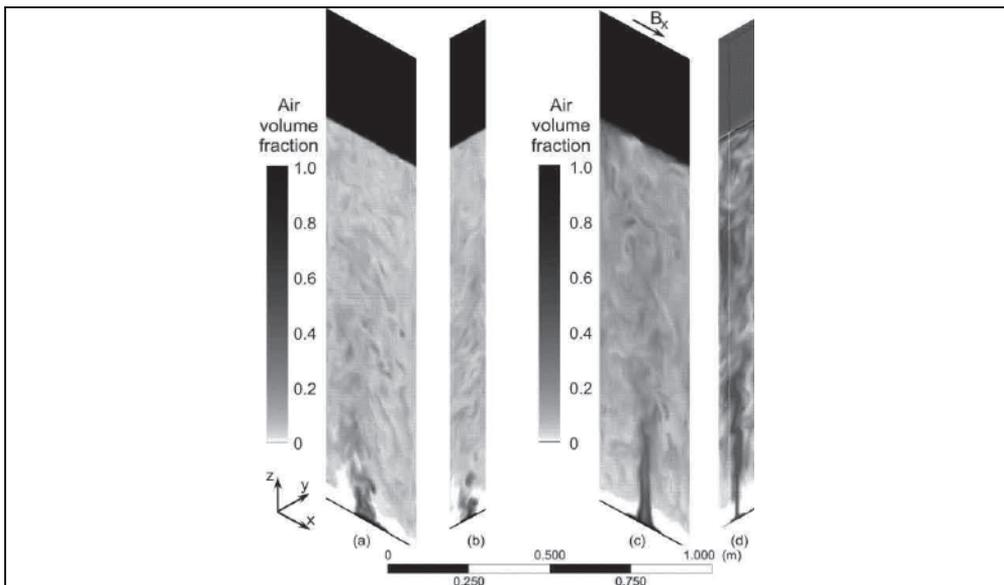
Fig. 1. Air-‘water-like’ liquid *RBR* – cross-sections: (a, c)  $y=0$  and (b, d)  $x=0$ .
