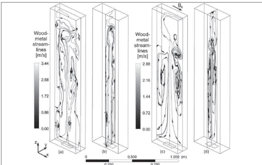
Fig. 3.  $N_2$ -Wood-metal RBR – cross-sections: (a, c)  $y=0$  and (b, d)  $x=0$ . Instantaneous (flow time  $t = 5$  s) Wood-metal streamlines in peripheral zone of container: (a, b) without magnetic field  $B = 0$ ; (c, d) with transversal external magnetic field  $B_x = 0.1$  T
