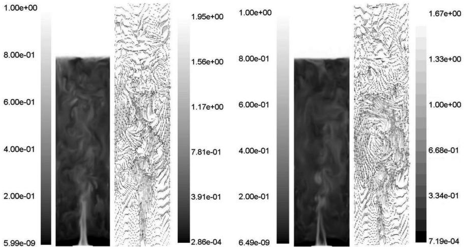
Figure 6. Rectangle bubble reactor. Horizontal  $B_x=0.1$  T (left) and vertical  $B_z=0.1$  T (right) magnetic field is “switched on” – vector of magnetic induction is parallel to the plane of figure. Instantaneous (flow time  $t = 20$  s) contours of gas volume fraction and velocity vectors of electrically conductive liquid (cross-sections  $y = 0$ ) obtained with *LES* model of turbulence. Gas velocity at inlet is  $0.5$  m/s (gas mass flow  $8.5 \cdot 10^{-3}$  kg/s).
