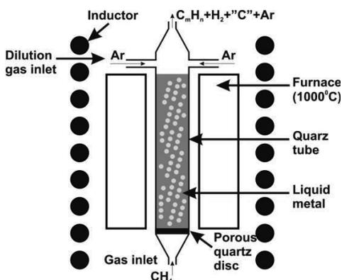
Figure 1. Liquid metal bubble column for  $H_2$  production without  $CO_2$  emission
