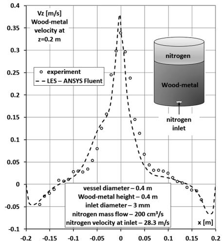
Figure 3. *Wood-metal* velocity vertical component for nitrogen–*Wood-metal CBR*. Comparison of experimental data [12] and computational results obtained with *LES* models of turbulence with *ANSYS Fluent*. Horizontal cross-section at height  $z = 0.2$  m; nitrogen velocity at inlet is 28.3 m/s
