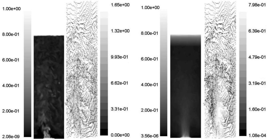
Figure 5. Rectangle bubble reactor. Magnetic field is “switched off” –  $B = 0$ . Instantaneous (flow time  $t = 20$  s) (left) and averaged (flow time  $t = 5$ – $20$  s) (right) contours of gas volume fraction and velocity vectors of electrically conductive liquid (cross-sections  $y = 0$ ) obtained with *LES* model of turbulence. Gas velocity at inlet is  $0.5$  m/s (gas mass flow  $8.5 \cdot 10^{-3}$  kg/s).
