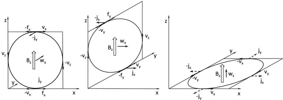
Figure 7. The scheme of vector fields in turbulent flow of electrically conductive liquid: liquid velocity is  $\vec{v}_l = \{v_x, v_y, v_z\}$ ; liquid velocity vortex is  $\vec{w}_l = \{w_x, w_y, w_z\}$ ; induction of external magnetic field is  $\vec{B}_0 = \{0, 0, B_z\}$ ; induced electrical current in liquid is  $\vec{j}_l = \{j_x, j_y, j_z\}$ ; EM force in liquid is  $\vec{f}_l = \{f_x, f_y, f_z\}$ .
