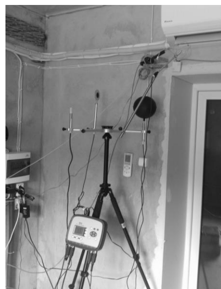
Fig. 4. Microclimate measuring device DeltaOHM HD 32.1 .
