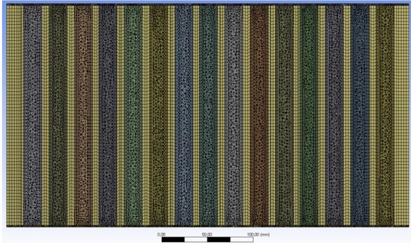
Fig. 3. Discretisation mesh in the middle cross-section of a modelled experimental block
