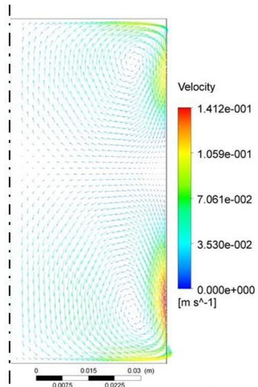
**Figure 2:** The average flow in half of symmetry plane of ICF (calculated using k- $\epsilon$  turbulence model).
