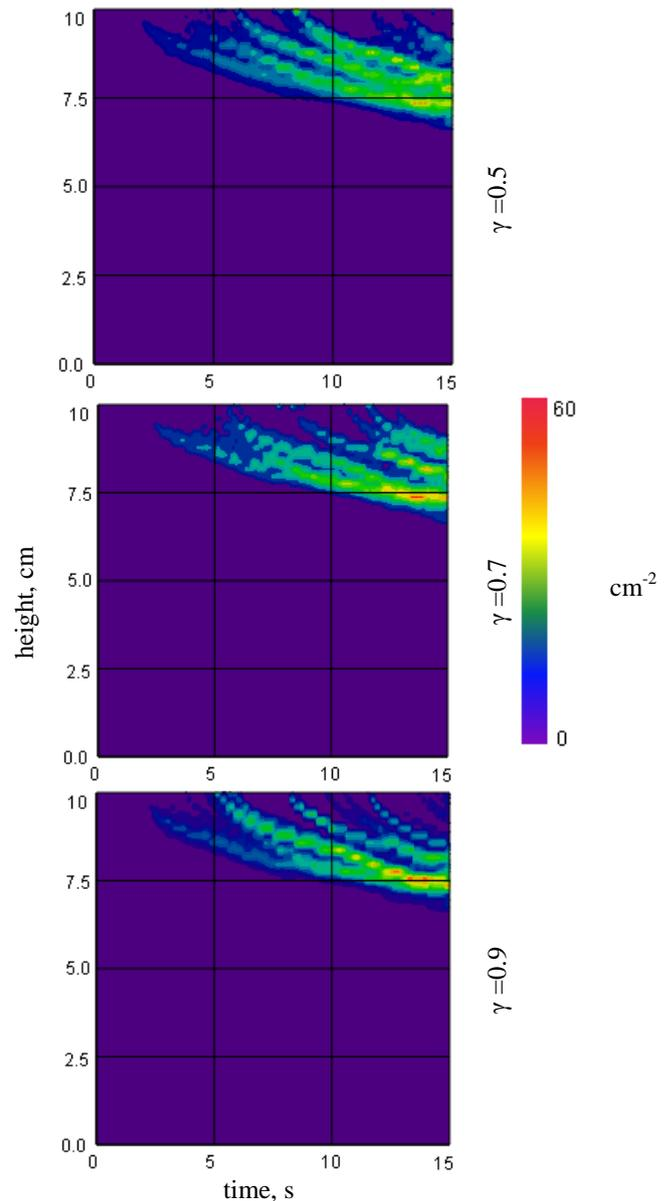
**Figure 8:** Time dependence of axial distribution of surface concentration ( $\text{cm}^{-2}$ ) of the deposited  $300 \mu\text{m}$  particles in ICF. Liquid-to-particle density rate is equal to 1.5. Parameter  $\gamma$  is the rate of semi-soft collision with the wall.
