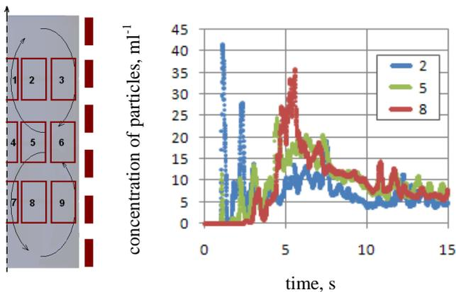
**Figure 5:** Dynamics of concentration of the particles in the different areas (simulated results). Areas are numbered on the sketch of the crucible (left image).
