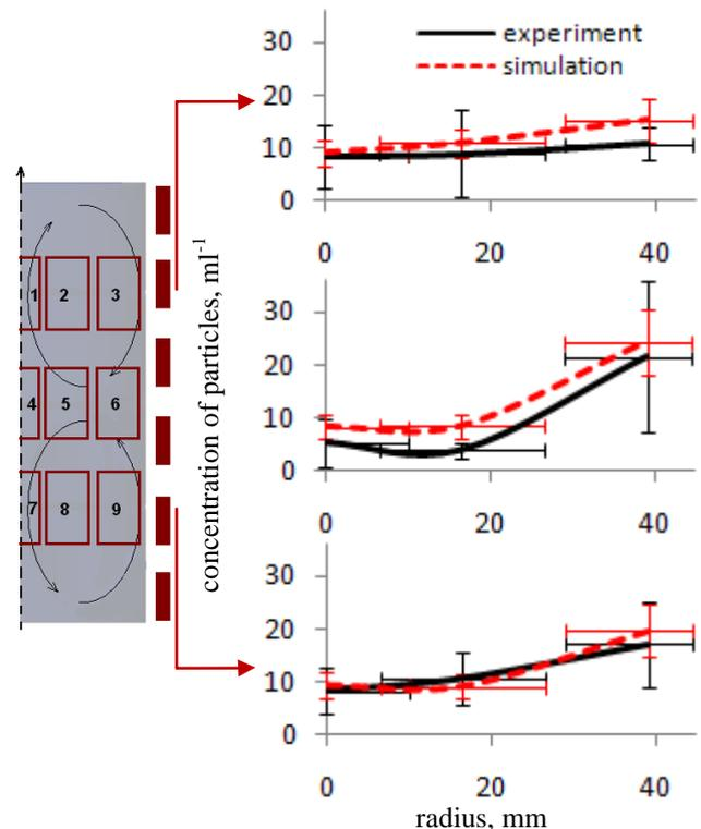
**Figure 6:** Experimental and numerical results of the concentration of solid  $300\pm 50\ \mu\text{m}$  inclusions in the flow of ICF at  $11\pm 2\ \text{s}$  from the beginning of stirring (quasi-stationary regime). Experimental samples were taken in the areas, they are marked with the red rectangles on the sketch of the crucible (left image).
