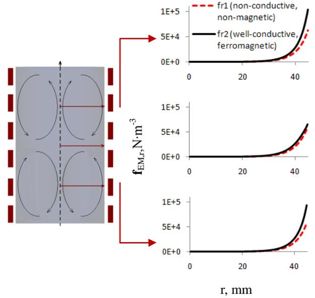
**Figure 3:** Magnitude of the EM force density (radial component) in the case of non-conductive & non-magnetic and well-conductive & ferromagnetic particles (see equations (3) and (5) respectively).
