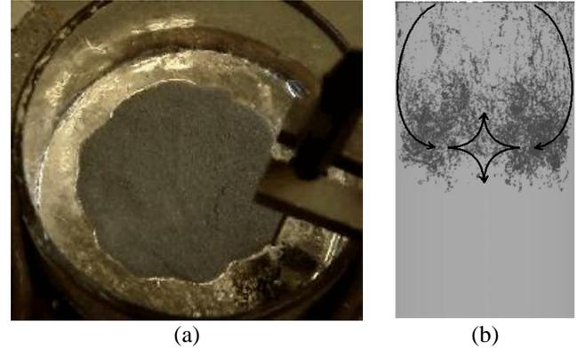
**Figure 4:** (a) Solid inclusions on the top surface of the melt in the laboratory ICF – initial position; (b) the scheme of motion of the inclusions from the initial position on the surface (vertical cross section of the crucible, simulated result).
