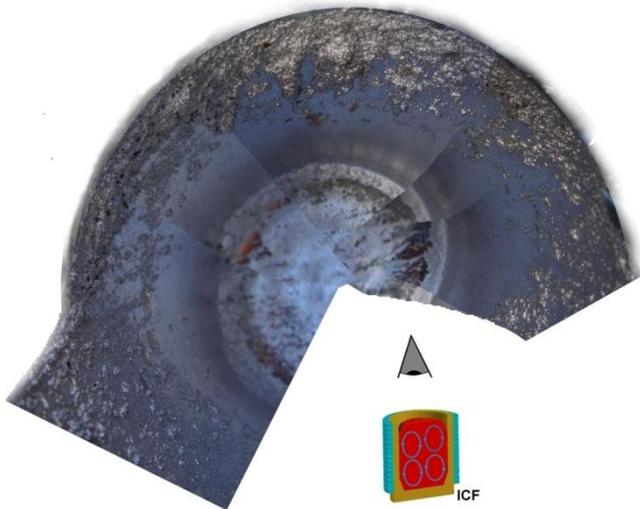
**Figure 7:** Deposition formation of iron particles on the walls of the experimental crucible. The ICF was drained after the experiment. This image is made from several photos of the crucible, viewing it from the top to the bottom.
