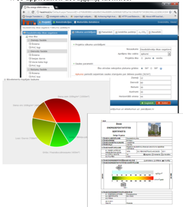
Fig. 1 Different features of HeatMod6 application (data input and visualization, certificate printout, etc)
