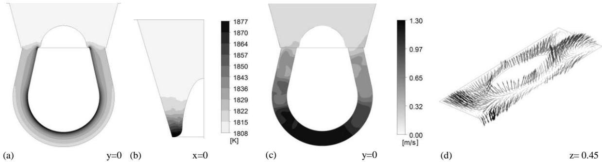
Fig. 3 Joule heat power (a, b), temperature field (c), velocity vectors (d) for cross-sections of Model (e) in Table 1
