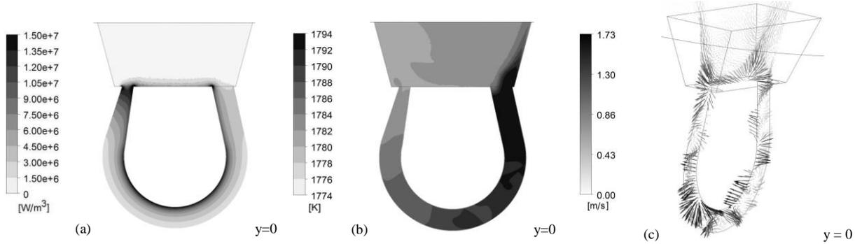
Fig. 2 Joule heat power (a), temperature field (b), velocity vectors (c) for cross-sections of Model (d) in Table 1
