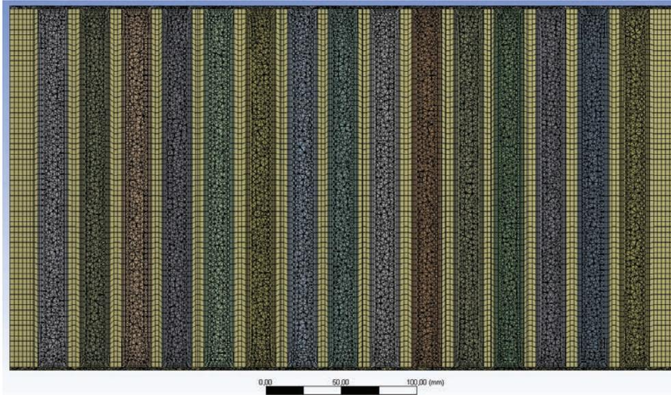
**Figure 3.** Discretisation mesh in the middle cross-section of a modelled experimental block
