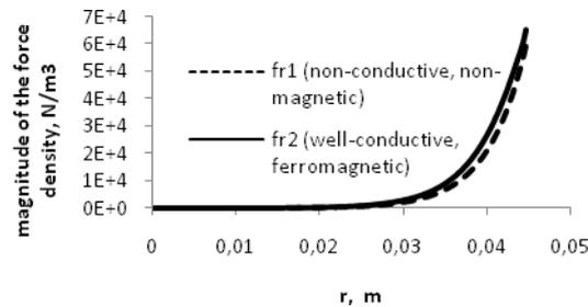
**Fig. 2** Magnitudes of the radial component of the EM force density for non-conductive & non-magnetic ( $f_1$ ) and for well-conductive & ferromagnetic ( $f_2$ ) particles at the middle of the small crucible.
