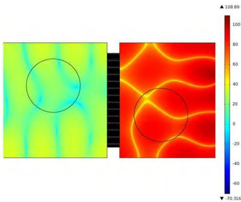
Figure 5. Sound pressure level in dB at 150Hz.
