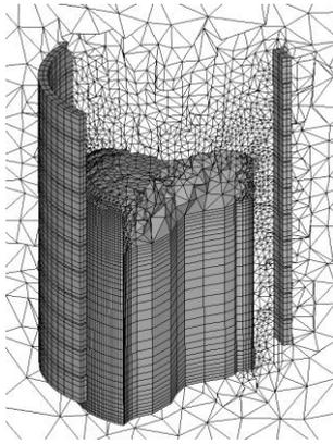
**Figure 6.** Free surface shape dependent 3D mesh for EM calculation.
