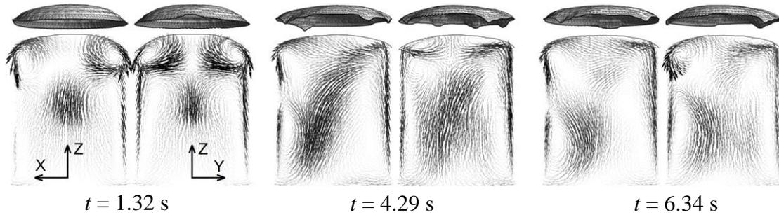
**Figure 8.** Flow pattern (0–0.4m/s) and free surface shapes at different time moments.
