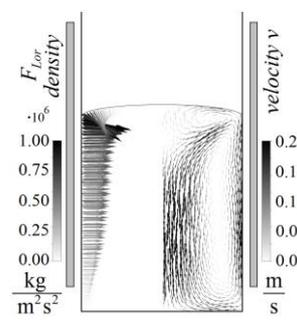
**Figure 3.**  $F_{Lor}$  density, steady state flow pattern and meniscus shape obtained with 2D HD model.
