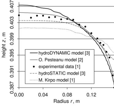
**Figure 2.** Comparison of 2D HD model results for quasi steady state meniscus shape to experimental data and other models.
