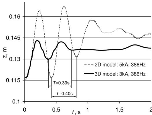
**Figure 11.** Comparison of free surface point oscillations on symmetry axis for 2D and 3D models.
