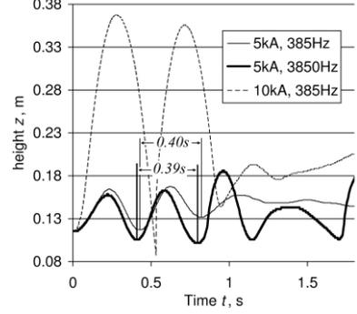
**Figure 4.** Free surface point oscillations on symmetry axis calculated with different current and frequency values.
