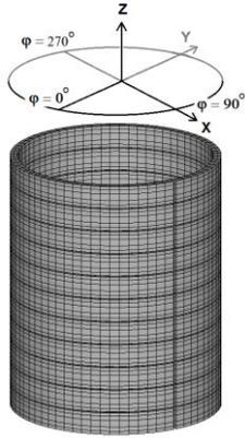
**Figure 7.** Separate inductor turns with gap for application of EM loads.
