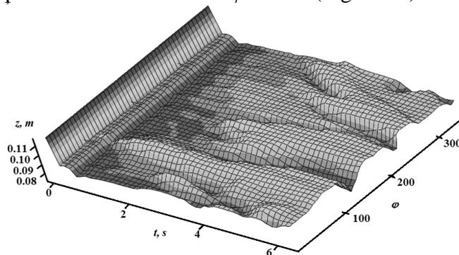
**Figure 9.** Surface plot representing the heights of meniscus perimeter points  $z$  as a function of time  $t$  and azimuthal angle  $\varphi$ .
