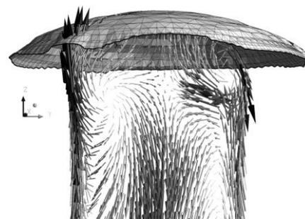
**Figure 10.** HD asymmetry ( $t = 2.5$  s) leads to upward flow along the walls and causes free surface perturbations.
