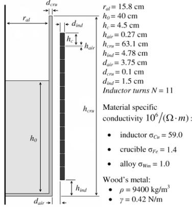
**Figure 1.** Geometry and material properties for ICF model.
