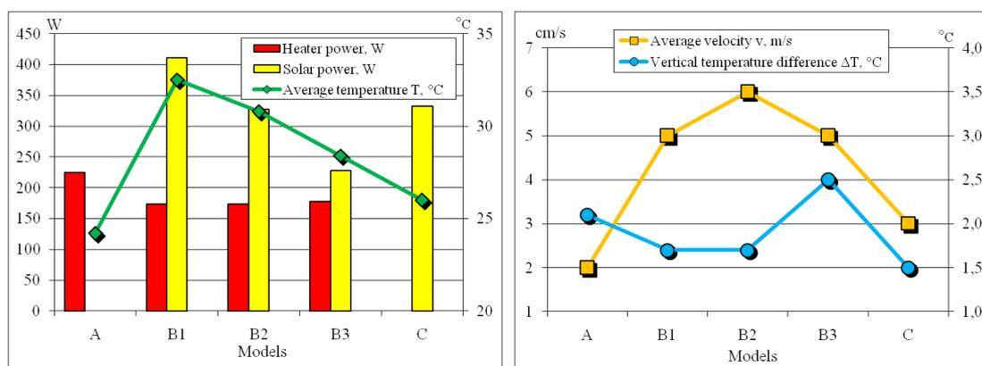
*Fig. 3. Heating powers, average temperature, vertical temperature difference and airflow velocity in the middle of the room for different variants.*
