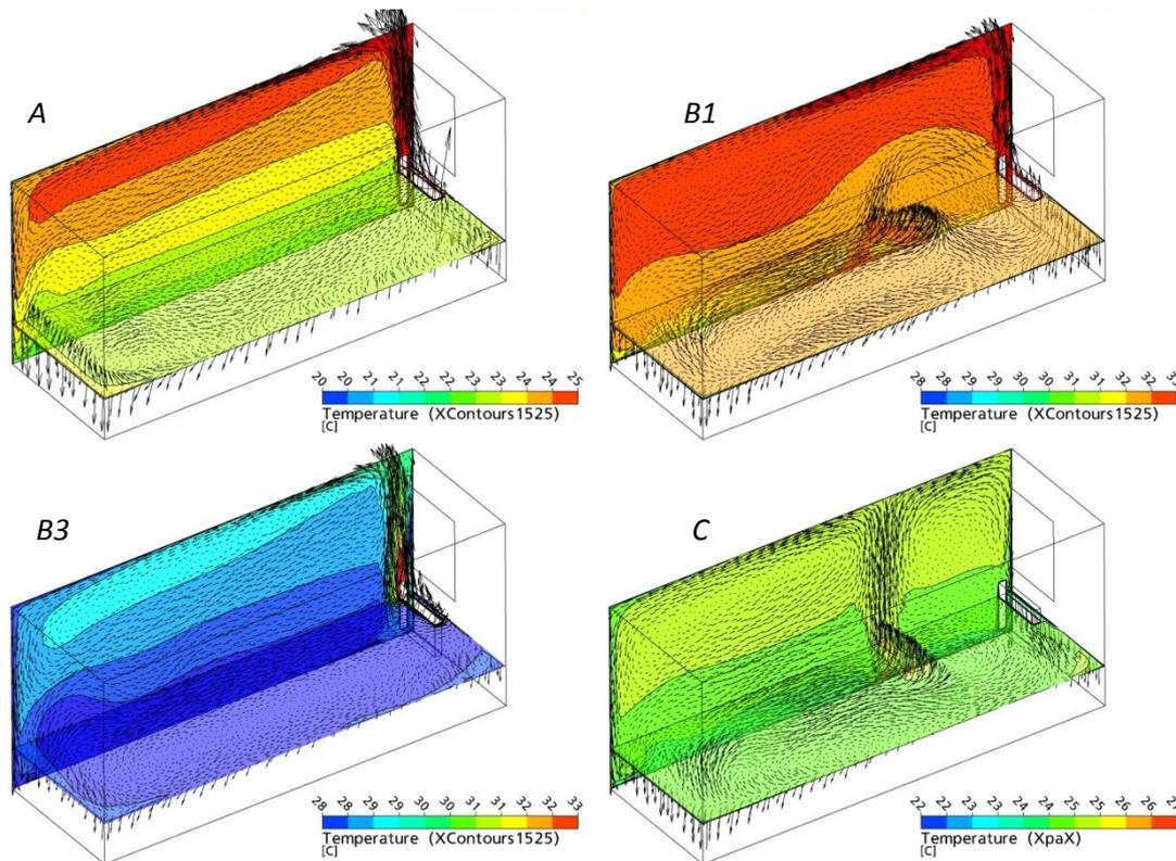
*Fig. 4. Velocity vector field and temperature contours in middle vertical cross-section and 0.5m height horizontal cross-section for variants A, B1, B3, C.*
