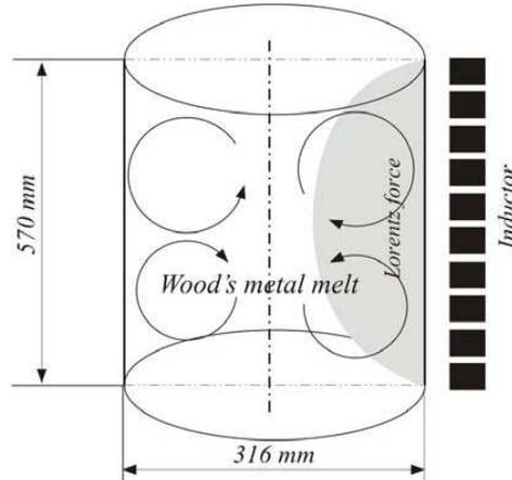
Figure 1. The design of ICF with the sketch of the typical vortices of the mean flow.
