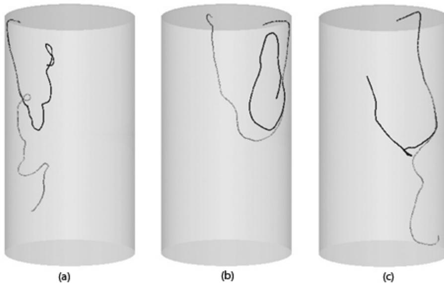
Figure 2. The trajectories of the particle taking into account different forces: dark colore trajectory – drag and EM forces; light colore trajectory – drag, EM, lift, acceleration and added mass forces.
