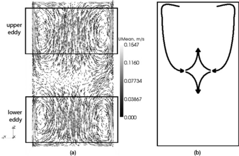
Figure 4. (a) – the average flow velocity in the central vertical plane in ICF; (b) – the scheme of the motion of the particle cloud in ICF.
