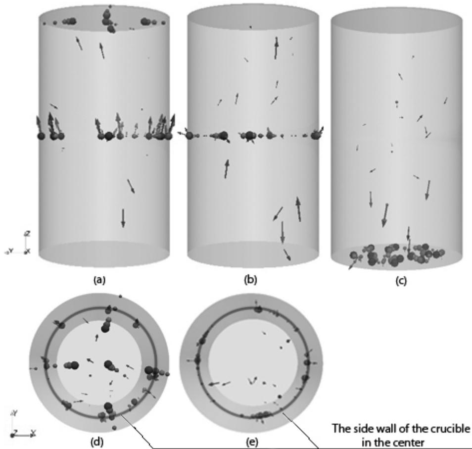
Figure 3. The positions of the particles in ICF after 7 s from the moment that they was input. The diameter of the particles ranges between 0.1 and 1.9 mm. (a), (d) -  $\rho_p = \rho_f / 1.5$ , (b), (e) -  $\rho_p = \rho_f$ , (c) -  $\rho_p = 1.5 \cdot \rho_f$ . The arrows show the direction and the magnitude of the momentary particle velocity at the 7 s. The images are drawn with respect to the optical perspective.
