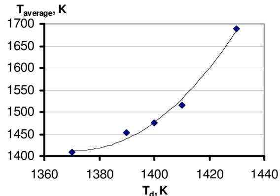
Fig. 5. Correlation between  $T_d$  and the average temperature in the melt:  $\varphi=0^\circ$
