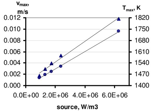
Fig. 3. Correlation of a Joule heat produced and the maximal velocity (*circles*) and temperature (*triangles*):  $\varphi=0^\circ$ ,  $1370\text{ K} < T_d < 1430\text{ K}$
