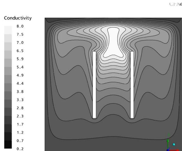
Fig. 2. Example of an electrical conductivity  $[S/m]$  distribution in the melt:  $T_d = 1410 K$
