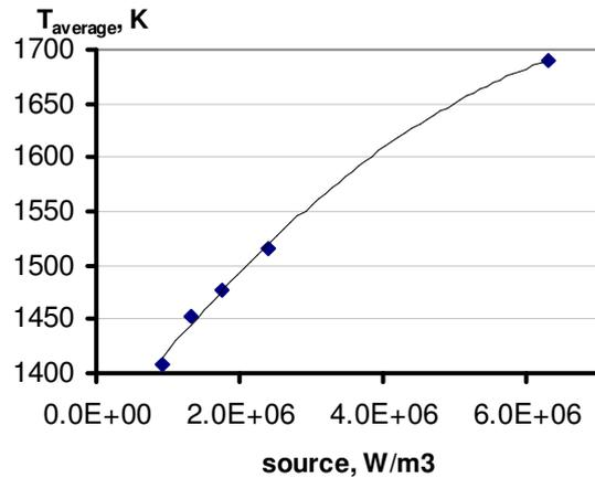
Fig. 4. Correlation of a Joule heat produced and the average temperature in the melt:  $\varphi=0^\circ$ ,  $1370\text{ K} < T_d < 1430\text{ K}$
