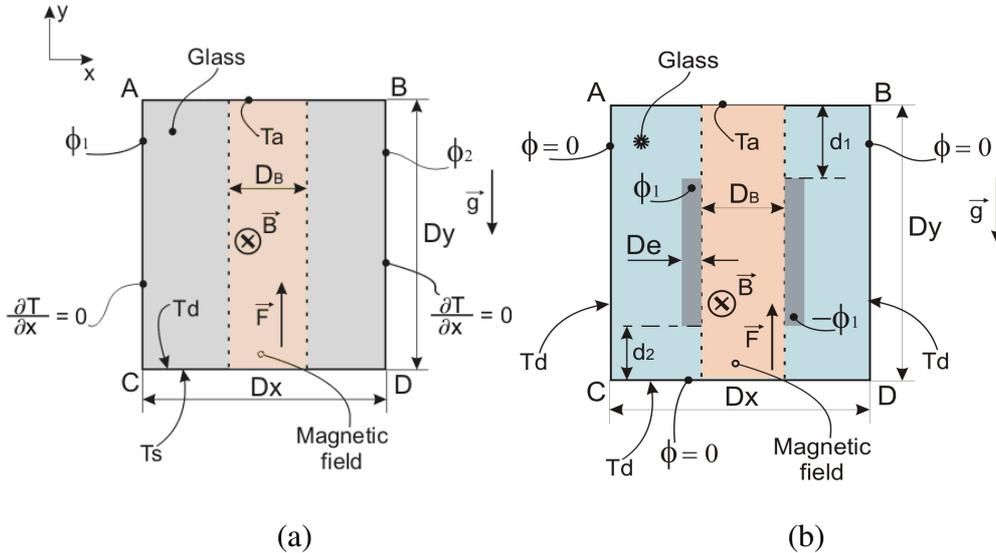
Fig. 1. 2D models for a stirring process of glass: a) without, b) with immersed electrodes.
