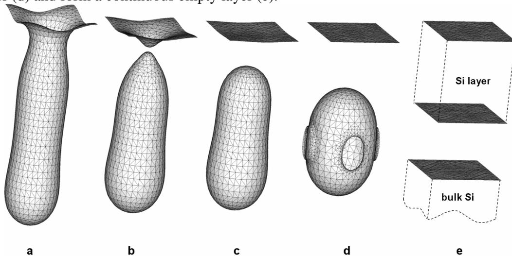
Figure 1. Time development of an SON layer represented by one trench out of an infinite calculated trench layer: neck formation (a), splicing of neck and bubble formation (b), bubble surface minimization (c), bubble joining with neighbouring bubbles (d), continuous layer formation (e).
