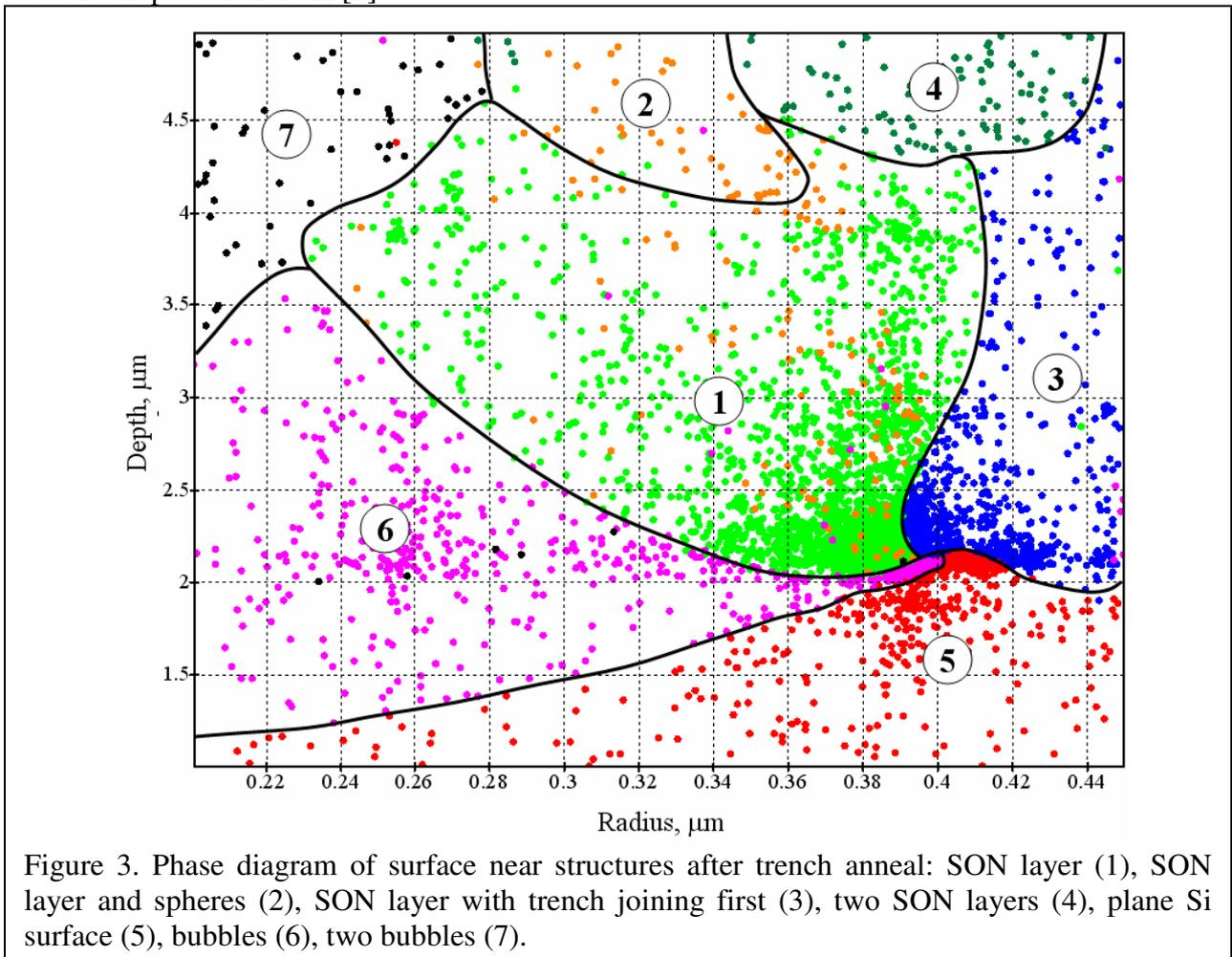
Figure 3. Phase diagram of surface near structures after trench anneal: SON layer (1), SON layer and spheres (2), SON layer with trench joining first (3), two SON layers (4), plane Si surface (5), bubbles (6), two bubbles (7).
