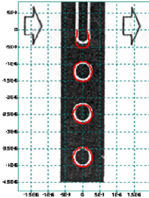
Figure 2. Comparison of simulation results (lines) with experimental bubble shapes taken from [2].
