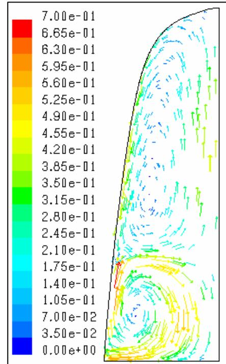
Fig. 2. Velocity vectors calculated with 2D RNG  $k-\varepsilon$  turbulence model [m/s]
