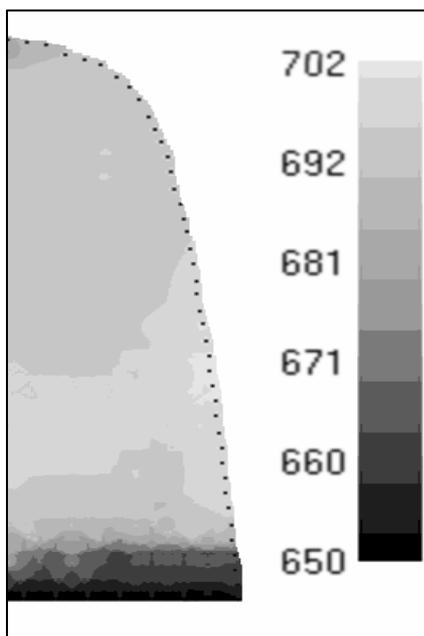
Fig. 1. Measured temperature distribution in aluminium melt in IFCC [°C]
