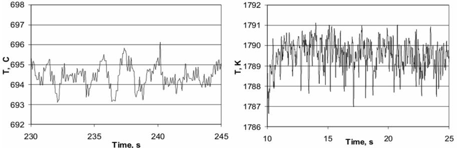
Figure 4: Temperature oscillations on the axis measured in aluminium (left) and calculated for TiAl alloy (right).
