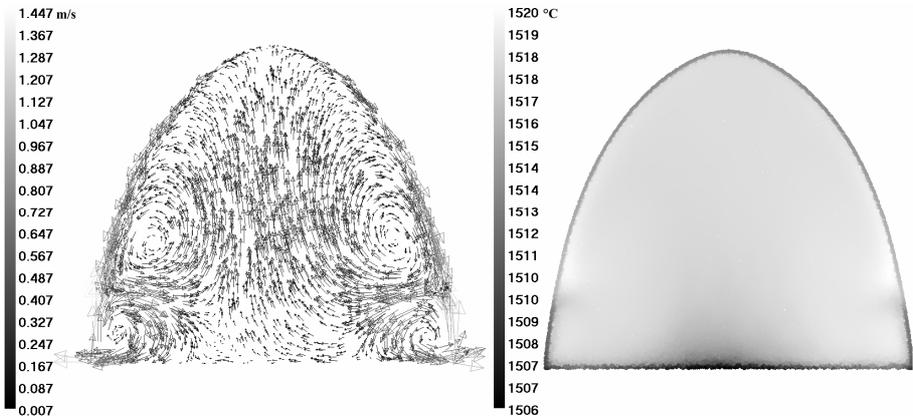
Figure 3: Time averaged velocity and temperature distribution in TiAl alloy.
