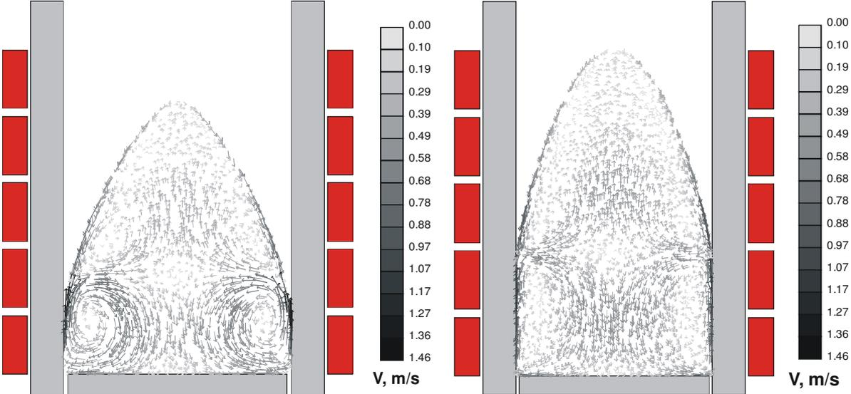
Fig. 5 Velocity vectors of TiAl melt in cold crucible with H/D ratios 1.20 (left) and 1.67 (right).
