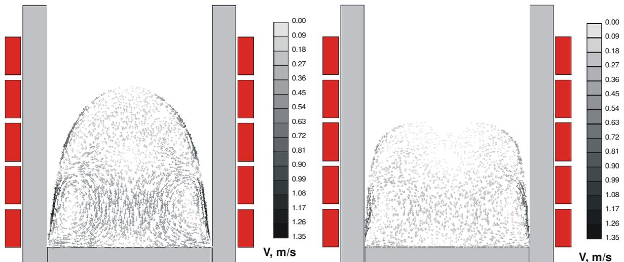
Fig. 6 Velocity vectors of TiAl melt in cold crucible with EM field frequency 5 kHz (left,  $H/D=0.99$ ) and 20 kHz (right,  $H/D=0.77$ ).
