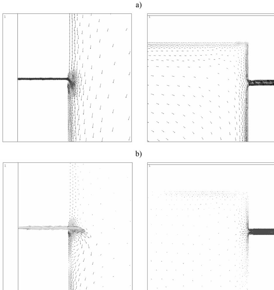
*Fig. 6. Vectors of airflow in openings of the room.
