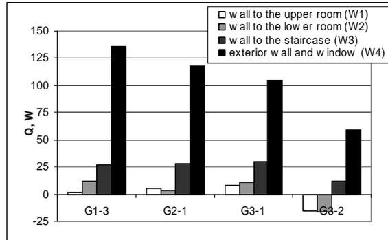
Fig. 10. Comparison of the conduction heat exchange for all boundary structures
