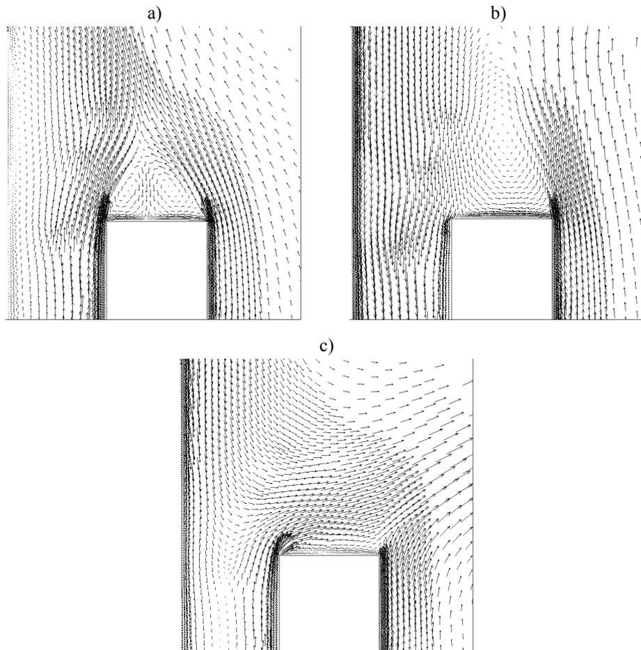
Fig. 4. Airflow vectors above the convector. Images *a*, *b*, *c* correspond to variants G1-1, G1-2, G1-3
