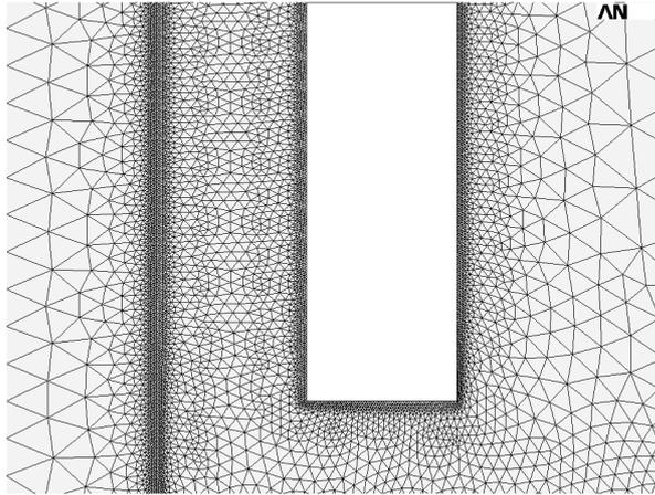
Fig. 2. Discretisation in the finite elements' method in the modelled corner of a room
