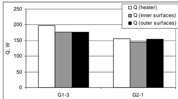
Fig. 9. Comparison of the conduction heat exchange for a confined room without convective losses
