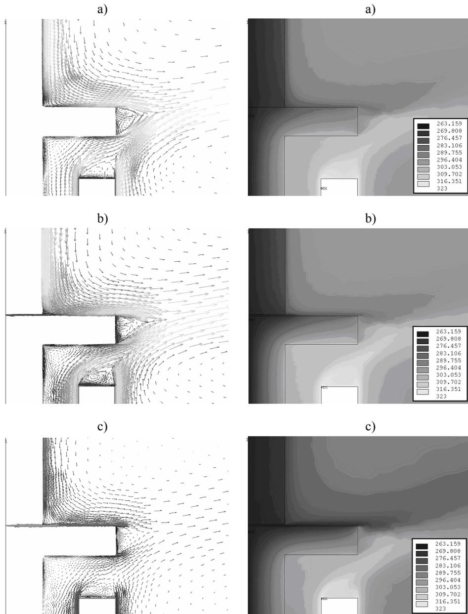
*Fig. 7* (left). Vectors of airflow above the convector.
