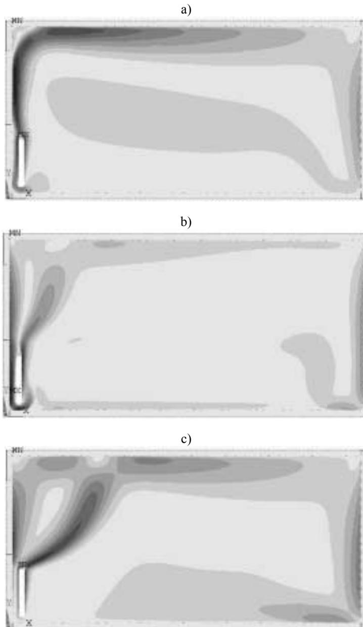
*Fig. 3. Stationary distribution of the velocity modulus in the modelled room. Images a, b, c correspond to variants G1-1, G1-2, G1-3.*
