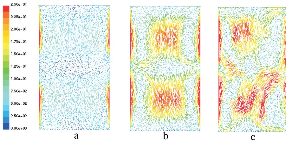
Figure 4: Flow pattern [m/s] after 2, 6 and 10 seconds of calculations
