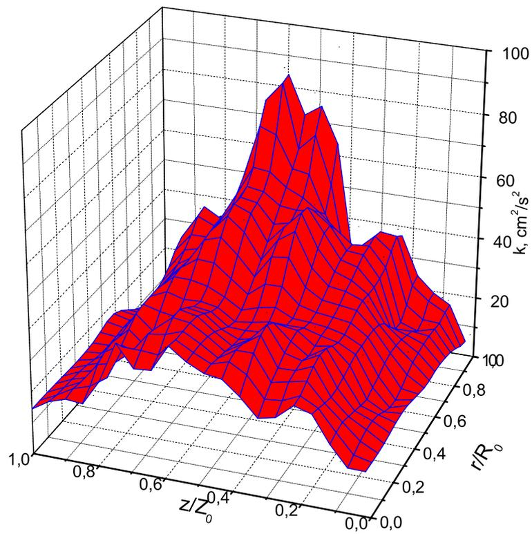
Figure 3: Kinetic energy of the oscillations measured in model furnace
