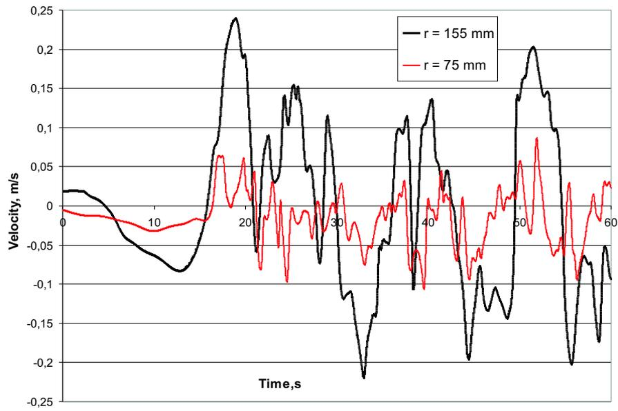
Figure 6: Axial velocity oscillations calculated with LES turbulence model on  $3.5 \cdot 10^6$  elements mesh
