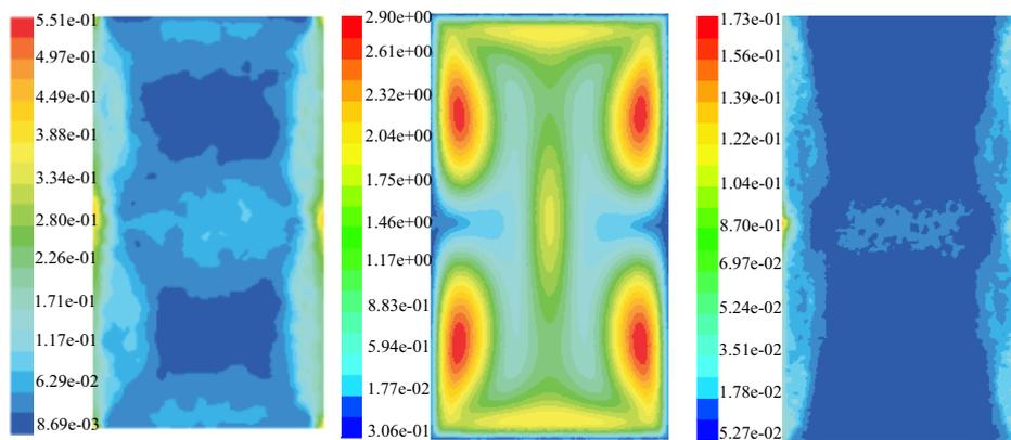
Figure 5: Turbulent viscosity distribution [ $kg/m \cdot s$ ] in case of  $k - \epsilon$  (middle) and LES 3D modeling on mesh with  $0.25 \cdot 10^6$  (left) and  $3.5 \cdot 10^6$  (right) elements
