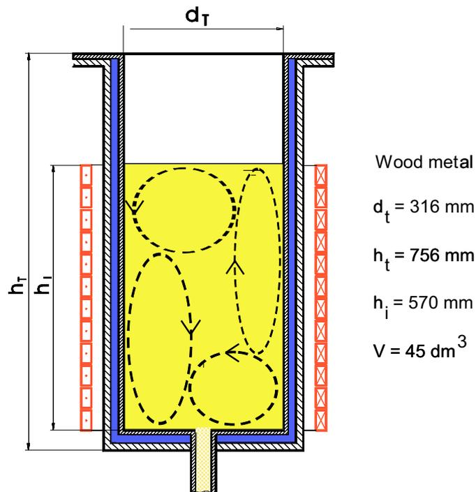
Figure 1: Experimental induction furnace used for 2D and 3D modeling. Characteristic flow directions and eddies' shapes are shown for the unstationary flow regime
