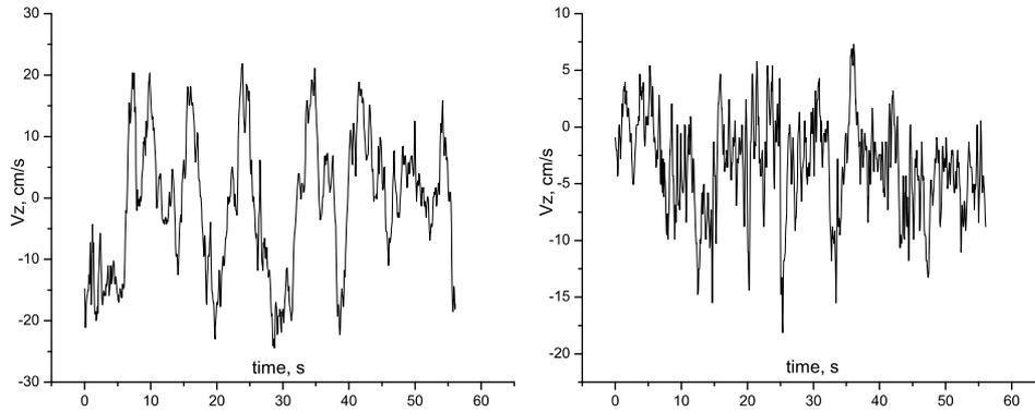
Figure 2: Measured axial velocity oscillations at the half-height of the inductor  $r=0.14\text{m}$  (left) and  $r=0.06\text{m}$  (right)
