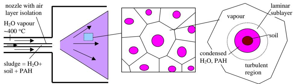
Fig. 1. Spraying of the sludge by superheated steam and steam stripping of PAH contaminated droplets
