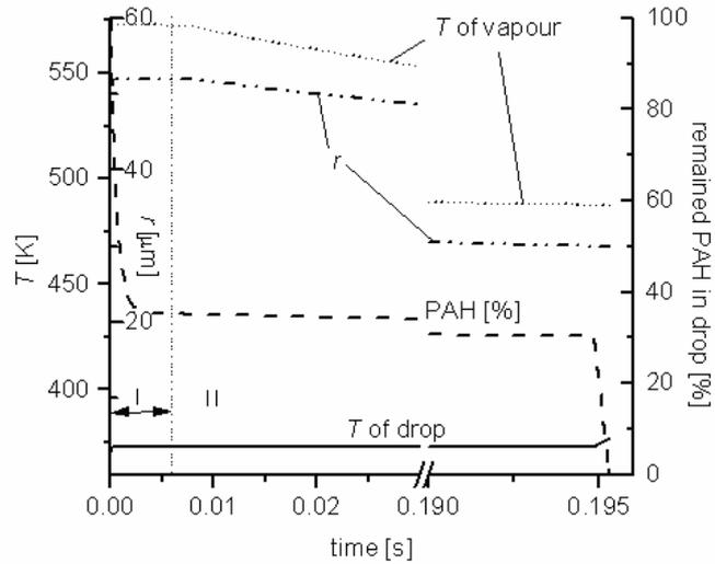
Fig. 4. Behaviour of the temperature of droplet and vapour, radius of droplet, and amount of PAH remained in the drop at steam stripping of pyrene. I – diffusion controlled approach, II – heat transfer controlled approach
