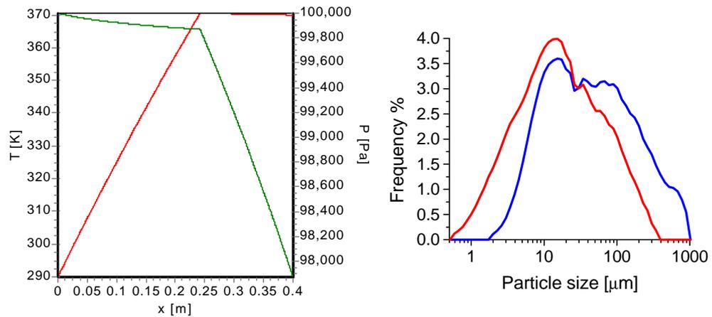
Fig. 2. Increase of temperature and decrease of pressure in a long Cu pipe with a layer of air insulation. The size of pipe in the equipment is about 10 cm, ensuring that boiling of water does not start inside the pipe
