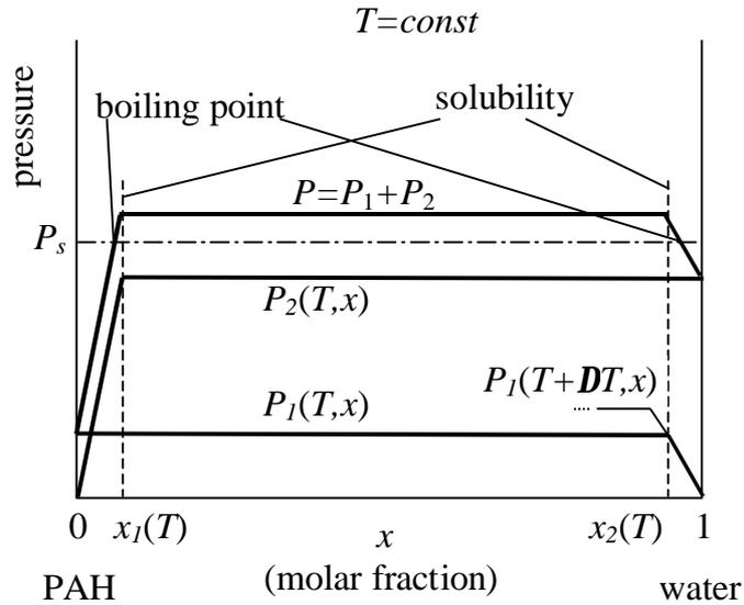
Fig. 4. Partial pressures of the components
