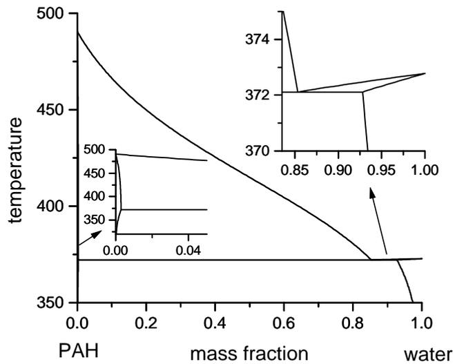
Fig. 5. Constructed phase diagram of naphthalene-water
