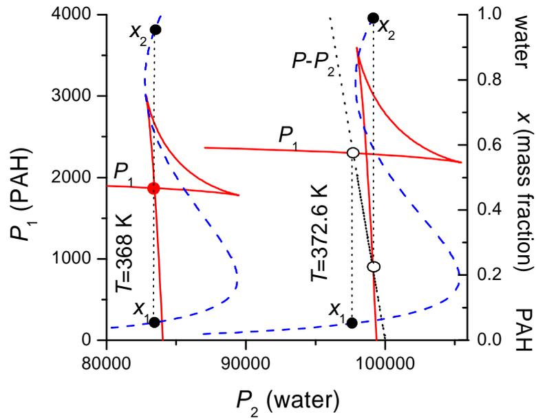
Fig. 10. Partial pressure of naphthalene vs. water (solid curve) at temperatures lower and higher than  $T_c$ . Dashed curve – mass fraction of water.  $x_1, x_2$ : phase transition points
