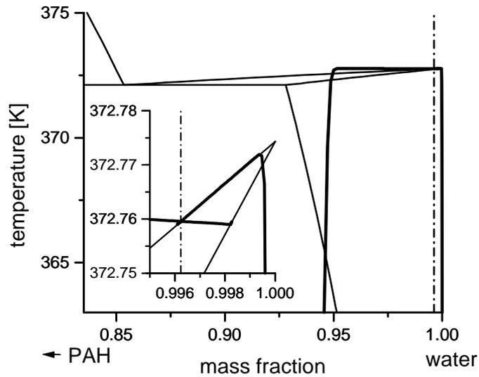
Fig. 6. Dynamics of the stripping in phase diagram, Fig. 5. Thick curves correspond to droplet and vapour at surface temperature. Dot-dashed line – total mass fraction  $x_i$  in cell
