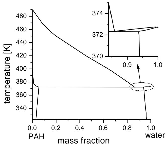
Fig. 11. Constructed phase diagram of naphthalene-water basing on partial pressures in Fig. 10
